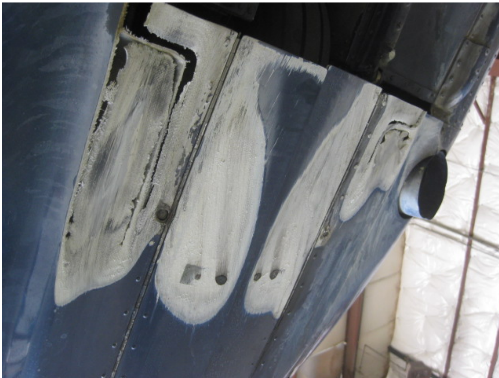
Photo 1 – Substantial Damage to Underside of Fuselage (Photo Courtesy of FAA)
