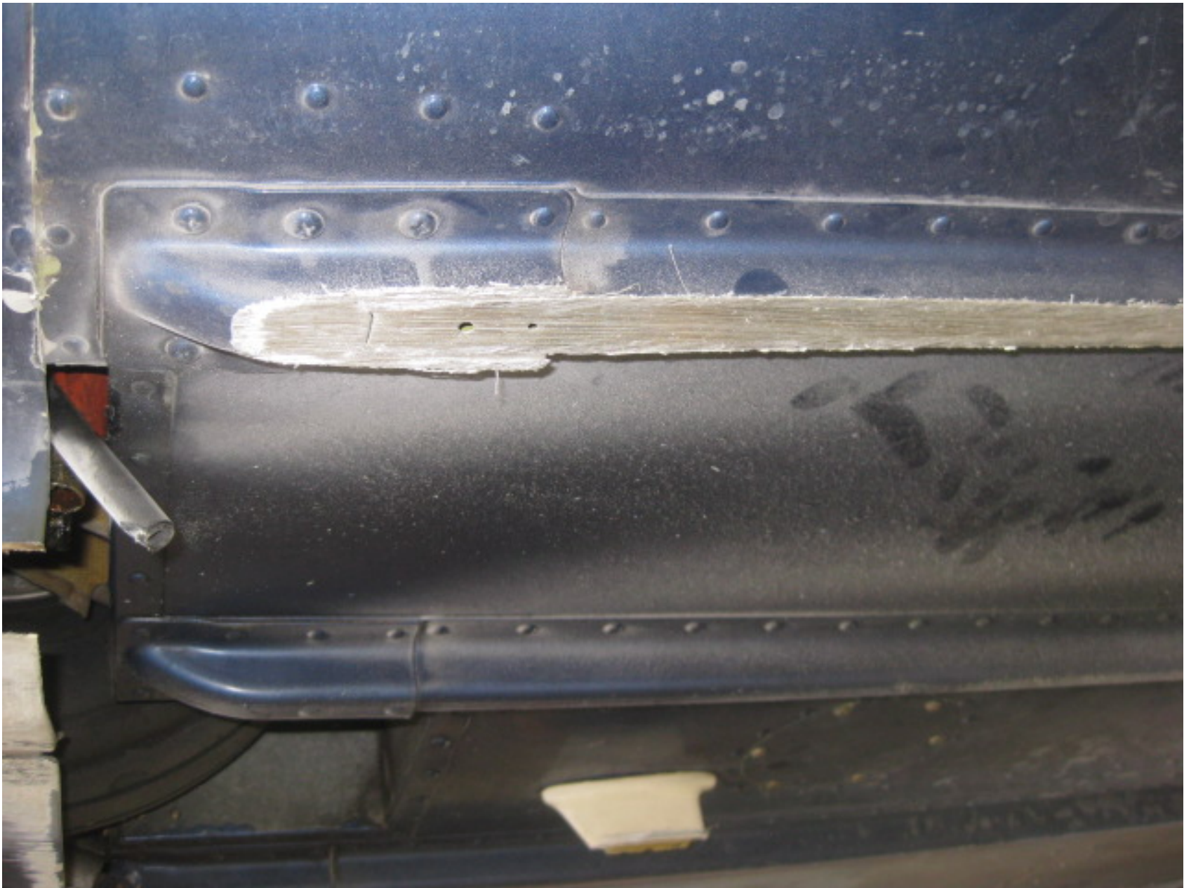
Photo 2 - Substantial Damage to Underside of Fuselage (Photo Courtesy of FAA)
