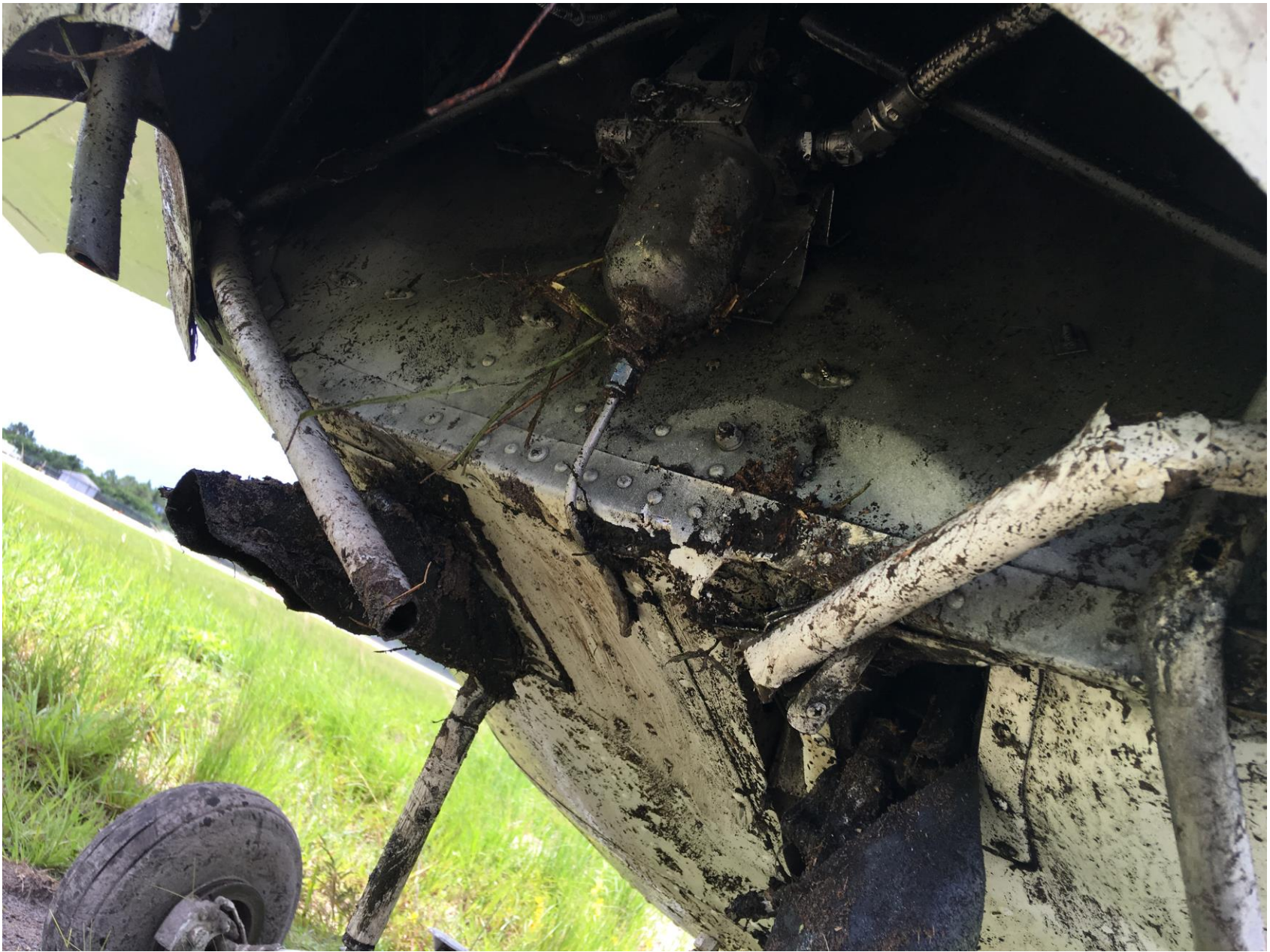
Photo 2 - View of firewall damage (photo courtesy of the FAA)
