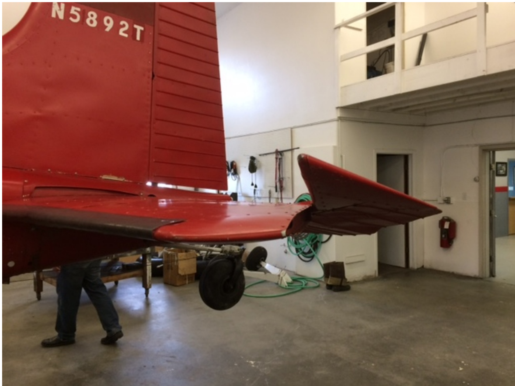
Photo 1 – View of damage to horizontal stabilizer and elevator (Courtesy of FAA)
