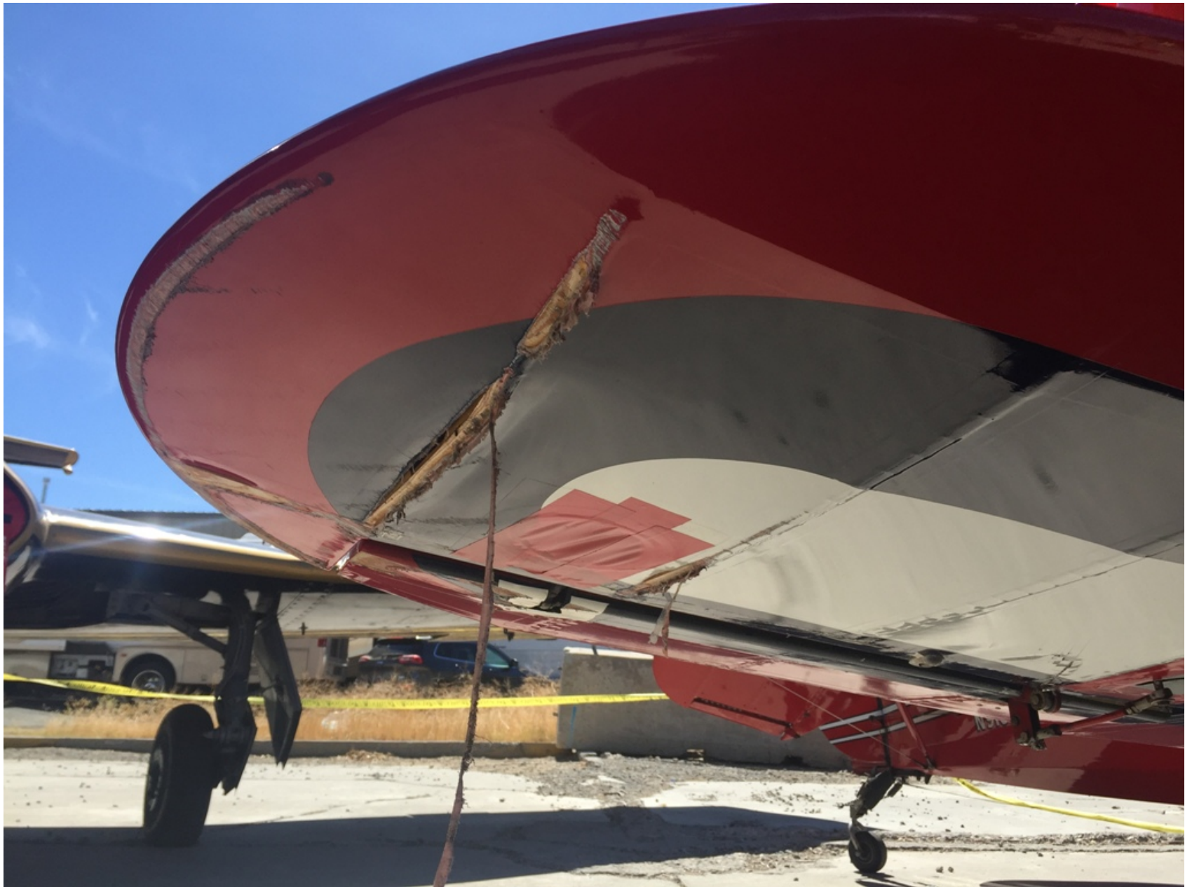
Photo 1 – View of damage to lower right wing ribs (Courtesy of FAA)
