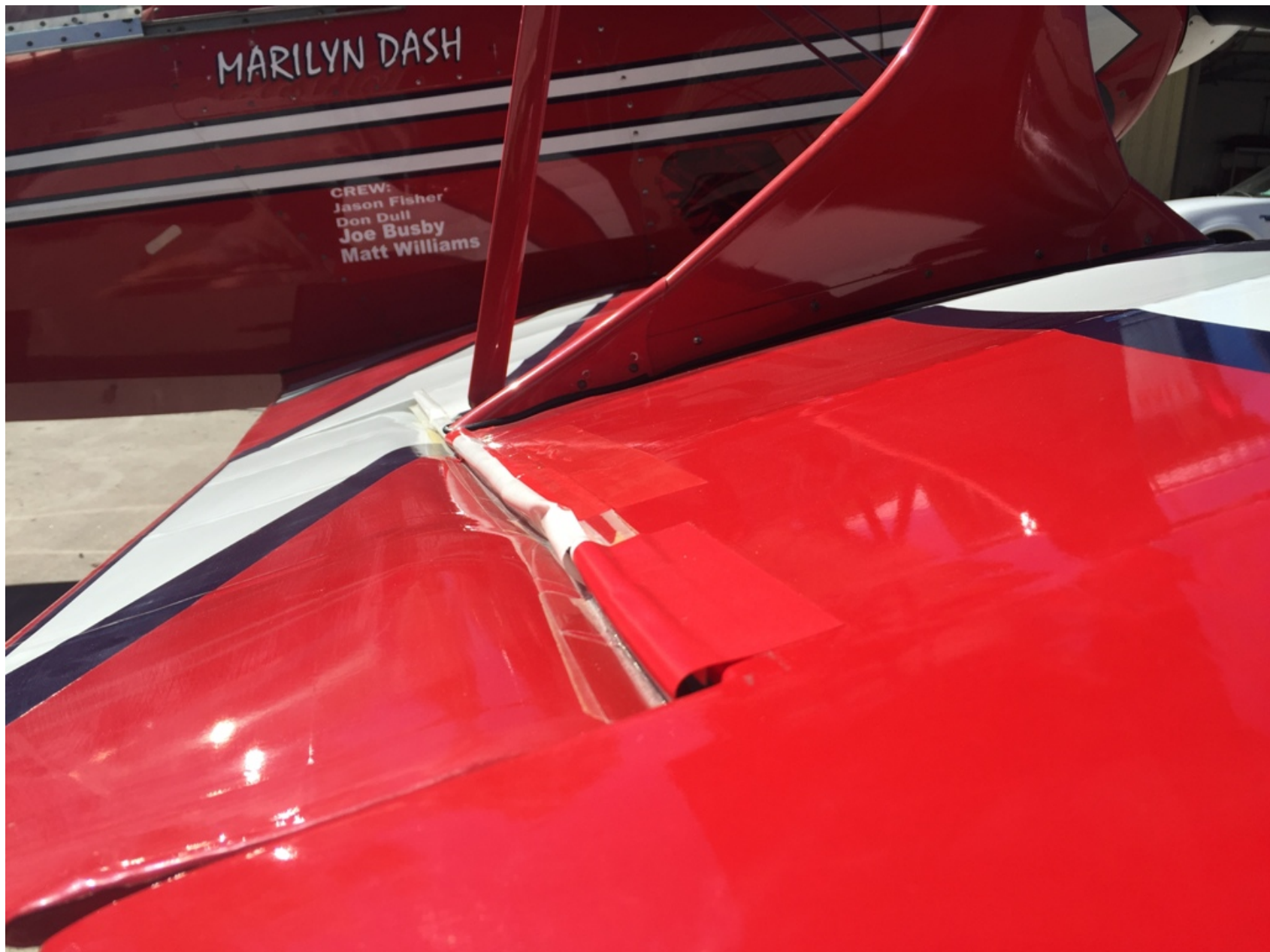
Photo 2 – View of damage to lower right wing (Courtesy of FAA)
