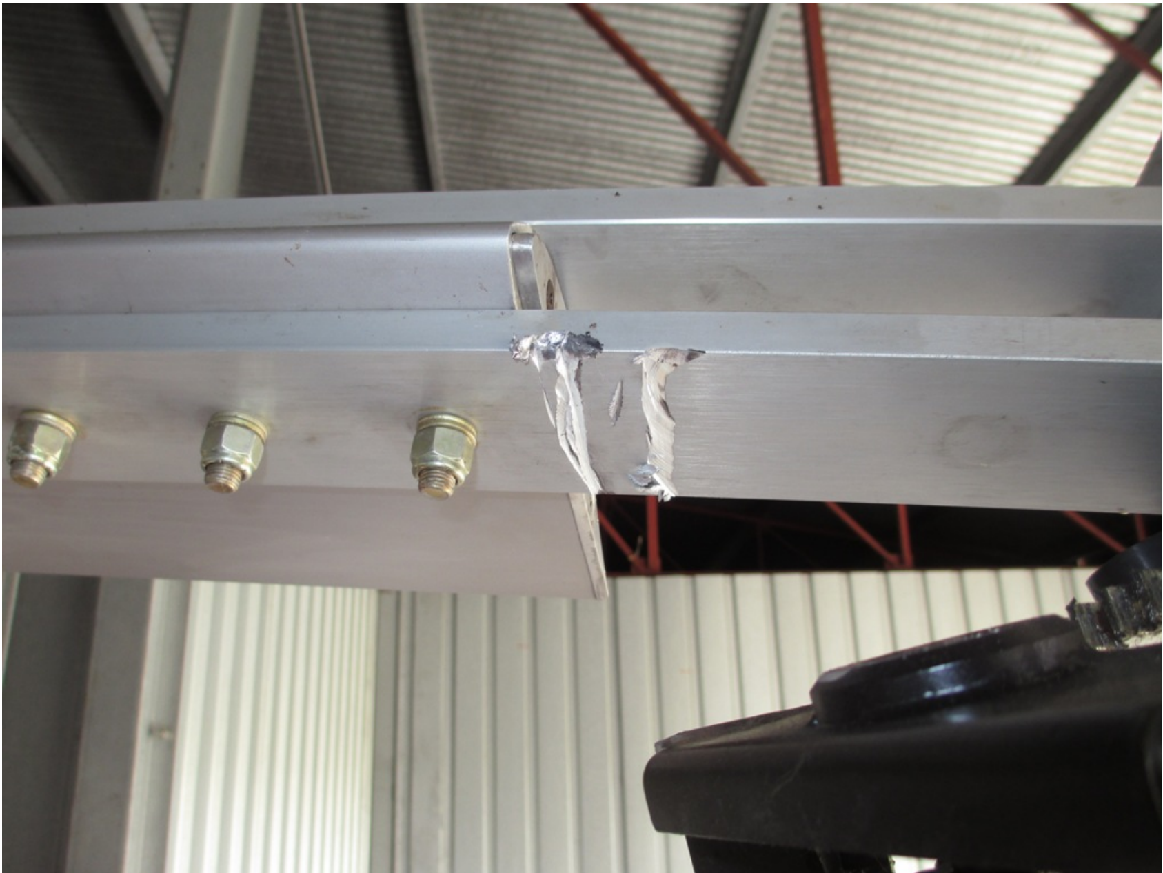
Photo 1 – View of damage to main rotor hub, blade grip (Courtesy of FAA)
