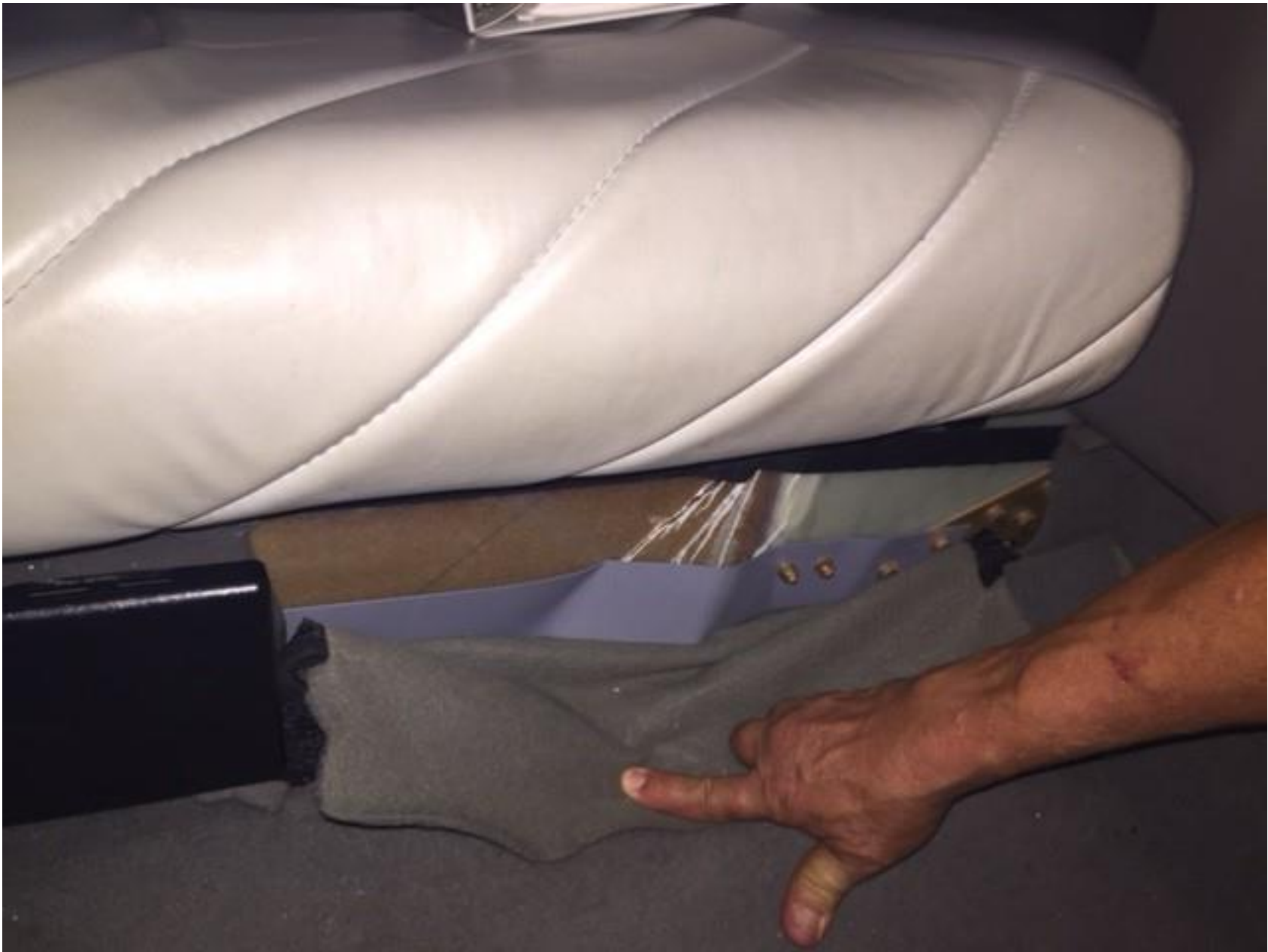
Photo 2 - View of wing root damage (photo courtesy of the FAA)
