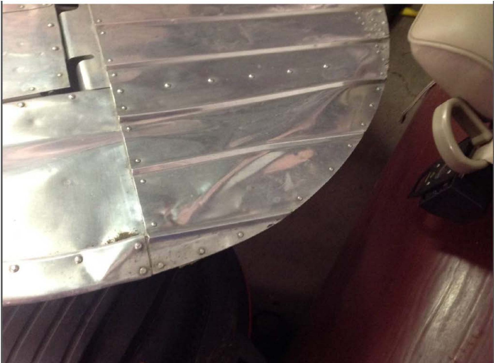
Photo 2 – View of damage to the elevator (Courtesy of FAA)
