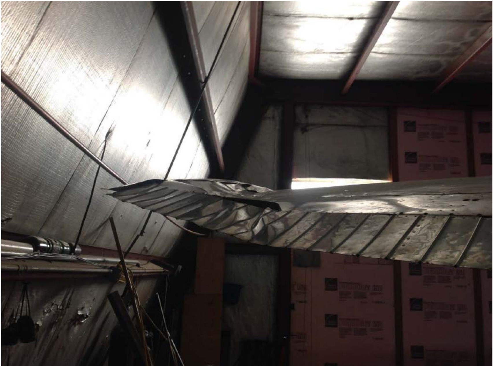
Photo 1 – View of substantial damage to left wing and aileron (Courtesy of FAA)
