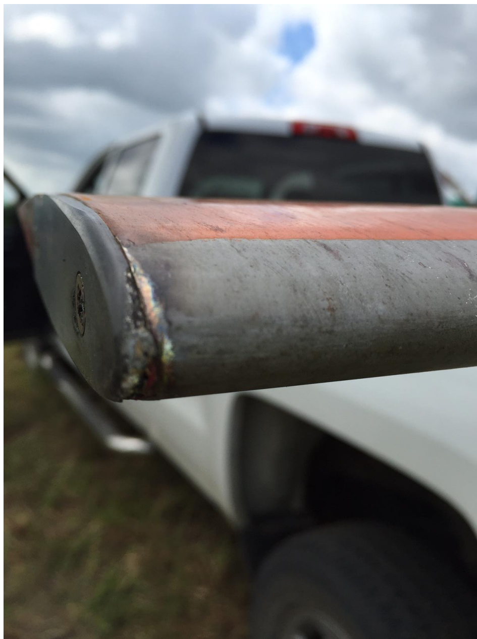
Photo 1 – View of damage to the leading edge of the main rotor blade (photo courtesy of the operator).
