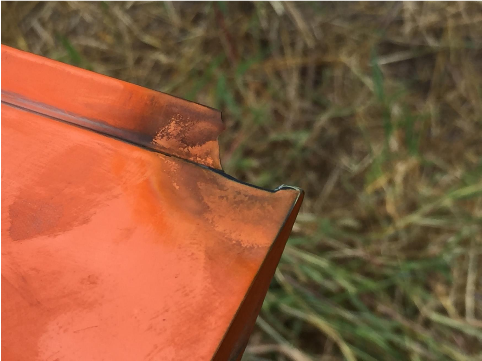
Photo 2 - View of damage to the trailing edge of the main rotor blade (photo courtesy of the operator).
