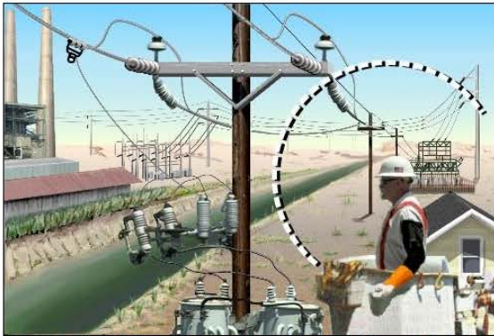
Figure 1. A schematic showing the minimum approach distance for a line worker. Depending on the voltage of the line (see the table below), a worker or a conductive object, must keep the minimum distance specified below between them and any energized part of the power line.
