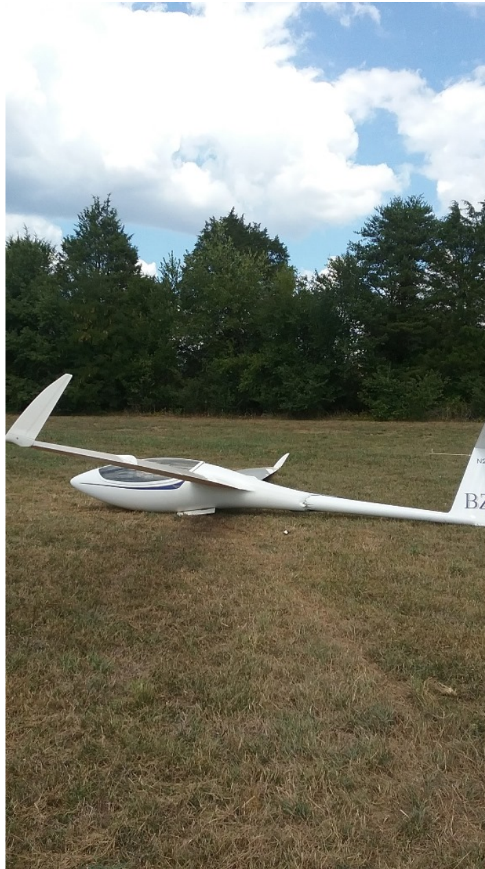
Photo 1 – View of substantial damage to tailboom (Courtesy of FAA)
