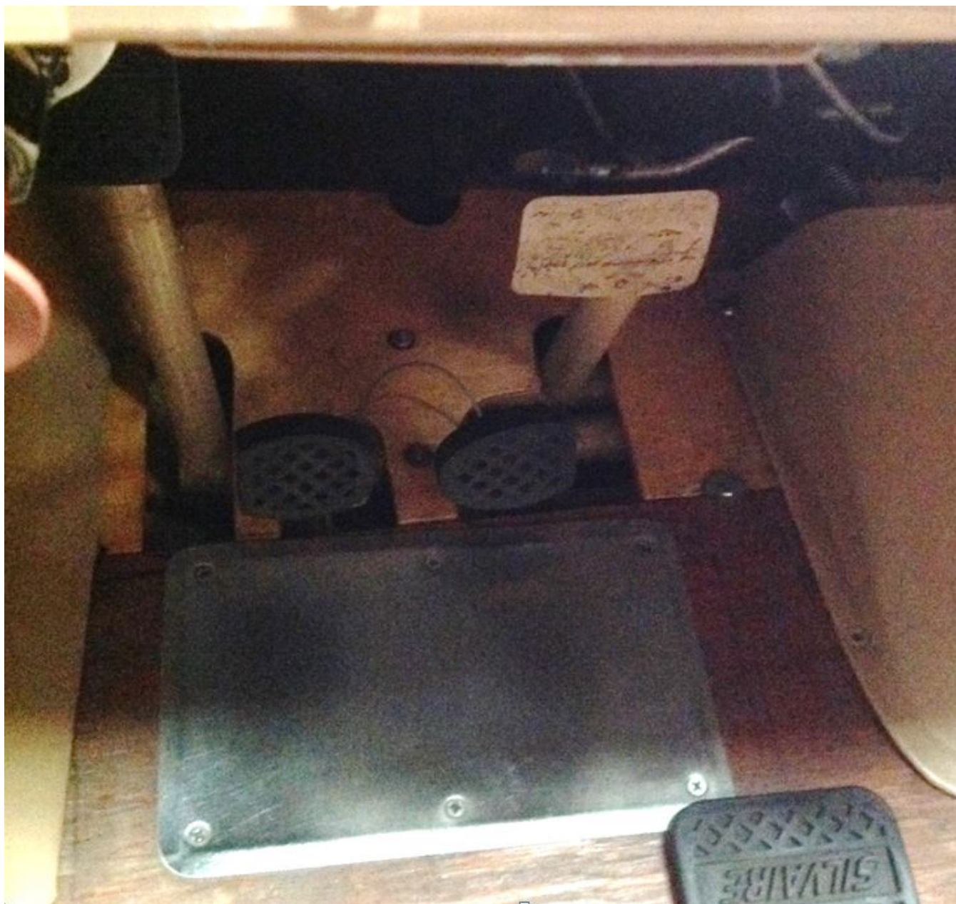
Photo 2 – Rubber Foot Pedal Next to Rudder Pedal (Photo Courtesy of Operator)
