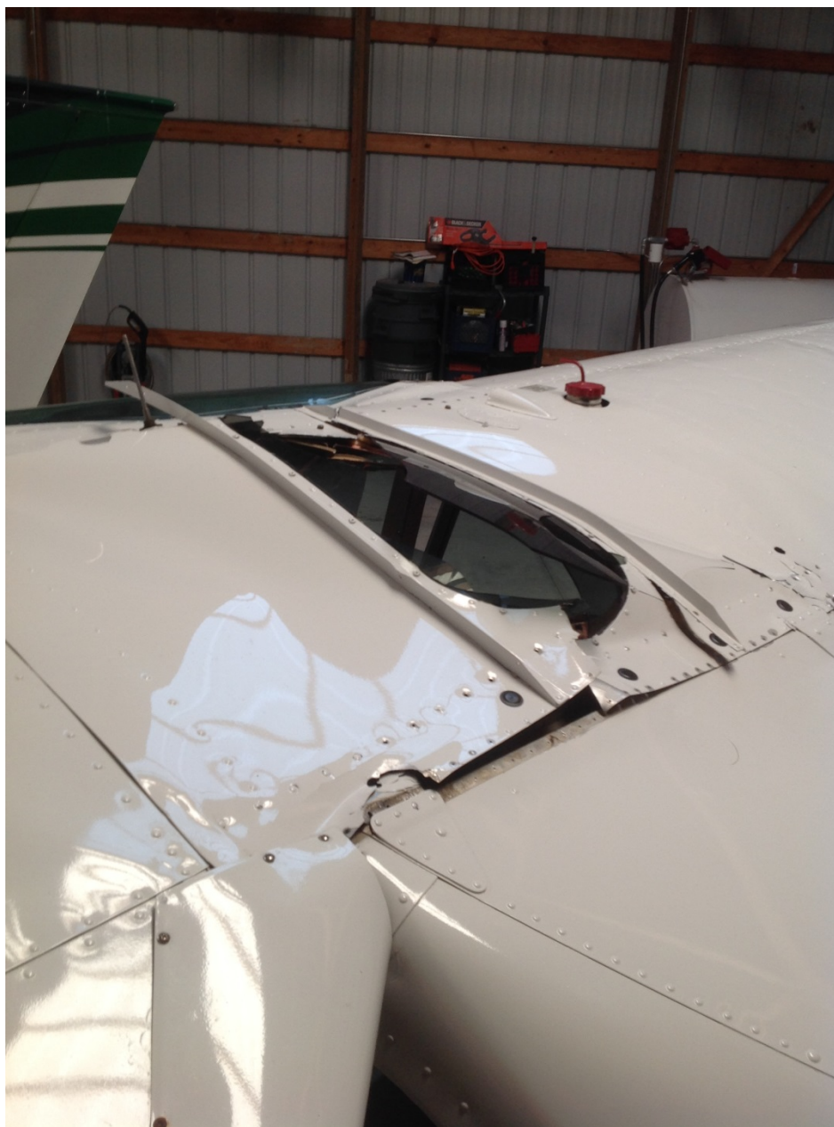
Photo 1 – Substantial Damage to Left Wing (Photo Courtesy of FAA)
