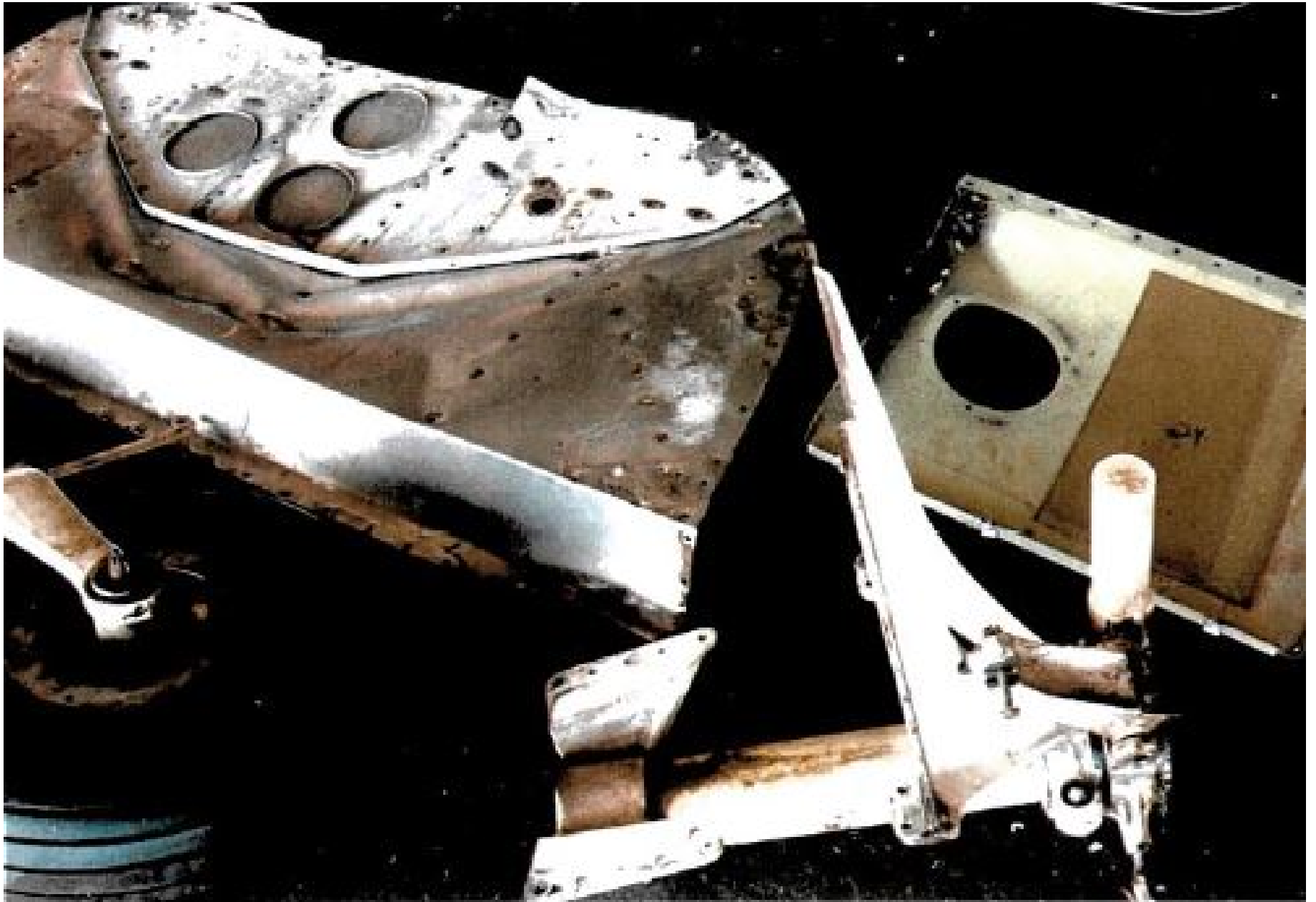
Photo 1 – Substantially Damaged Firewall (Photo Courtesy of FAA)
