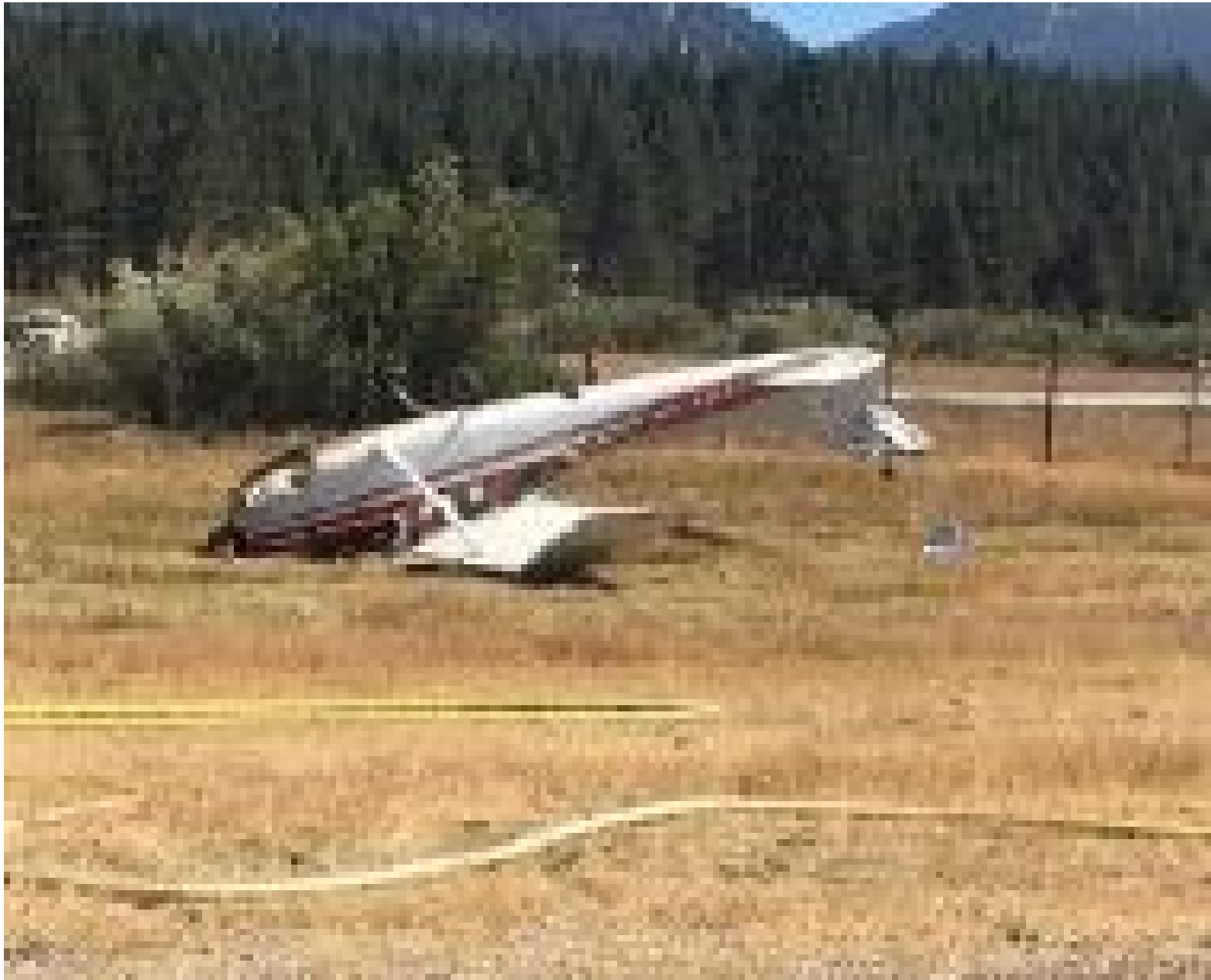
Photo 1 – Airplane Nosed Over Next to Runway (Photo Courtesy of FAA)
