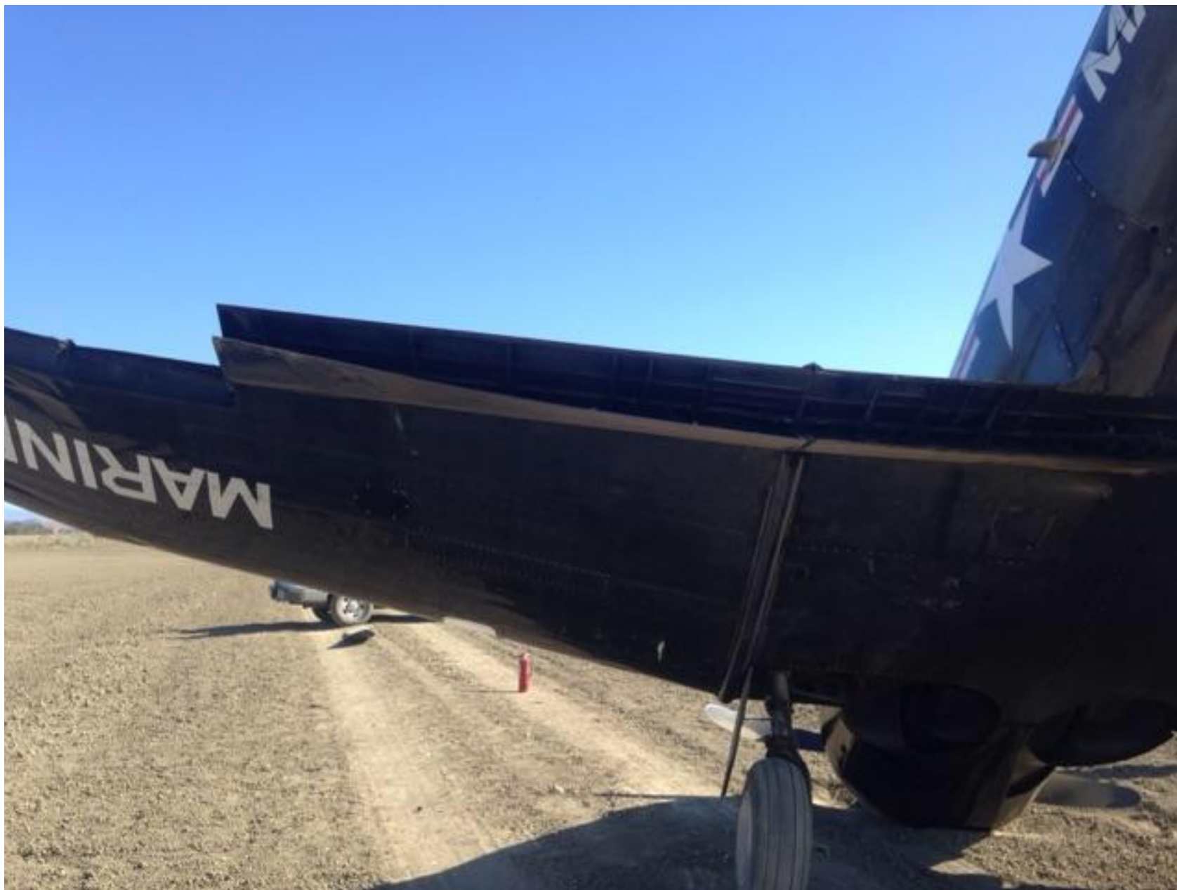
Photo 2 – Rear view of left wing damage (Photo courtesy of the NTSB)
