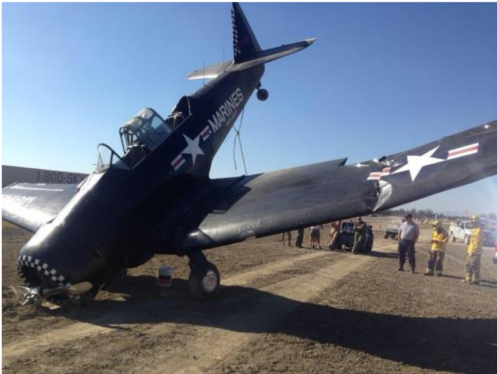
Photo 1 – Front left view of damage to wing and aileron area (Photo courtesy of the NTSB)
