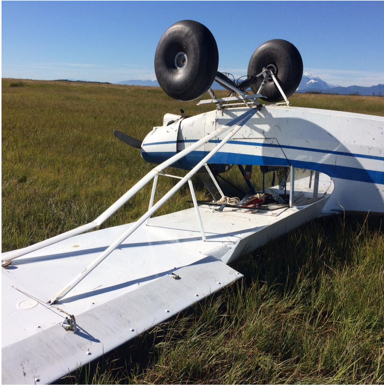
Photo 1 – View of damage to right wing strut (photo courtesy of the pilot)
