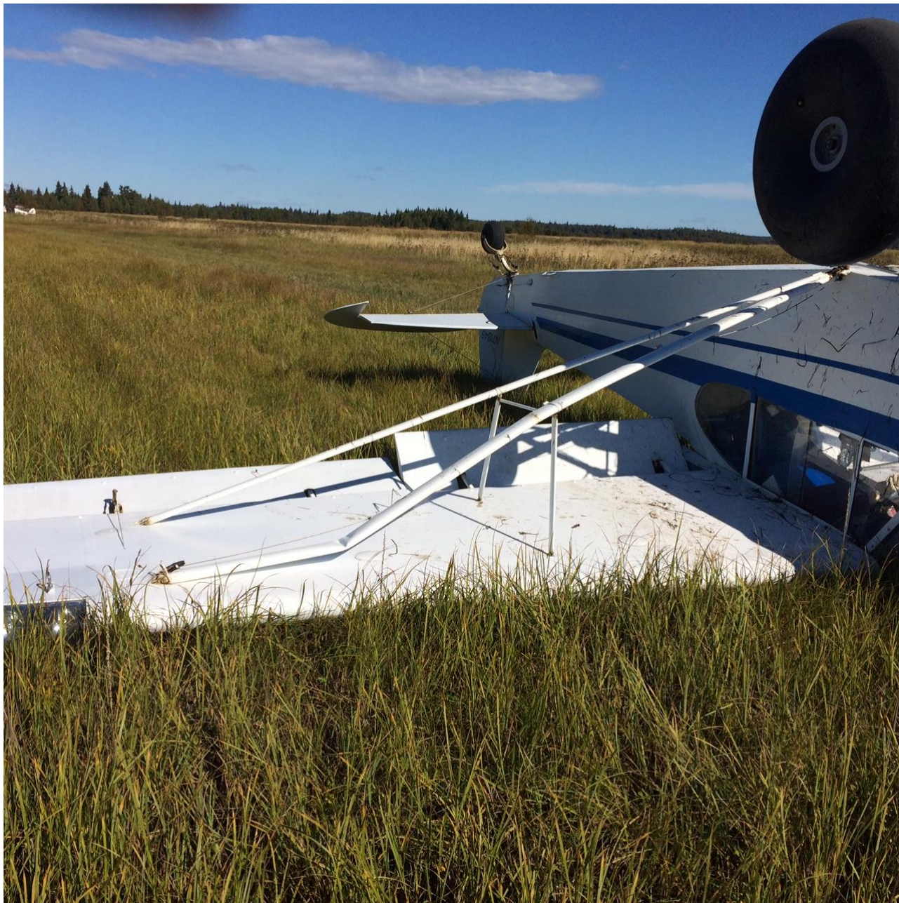
Photo 2 – View of damage to left wing strut (photo courtesy of the pilot)
