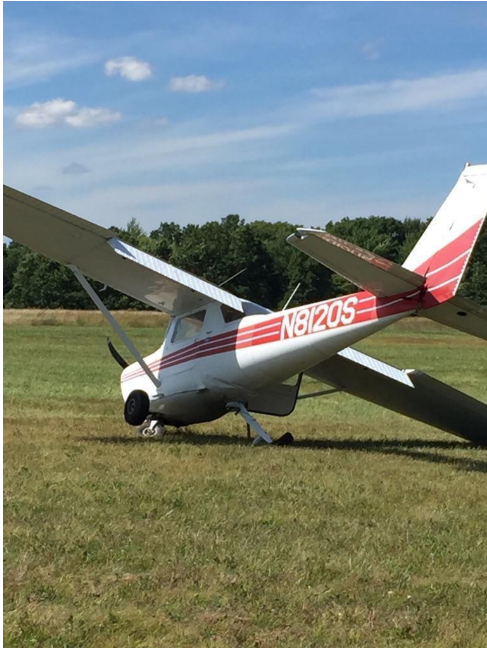
Photo 1 – View of substantial damage to the fuselage (photo courtesy of the FAA)
