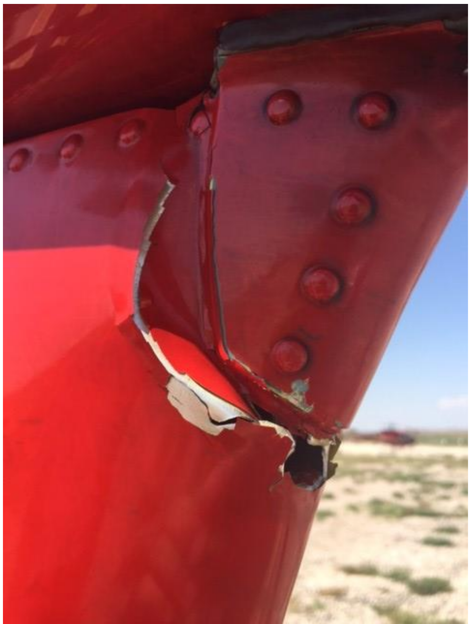
Photo 3 – Close up view of damage to the vertical stabilizer (Photo courtesy of the FAA)
