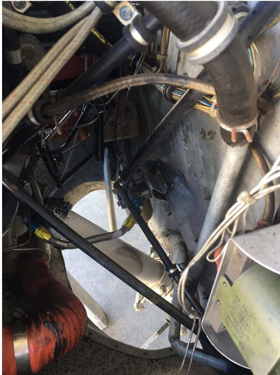
Photo 2 – View of damaged firewall (Courtesy of the FAA)
