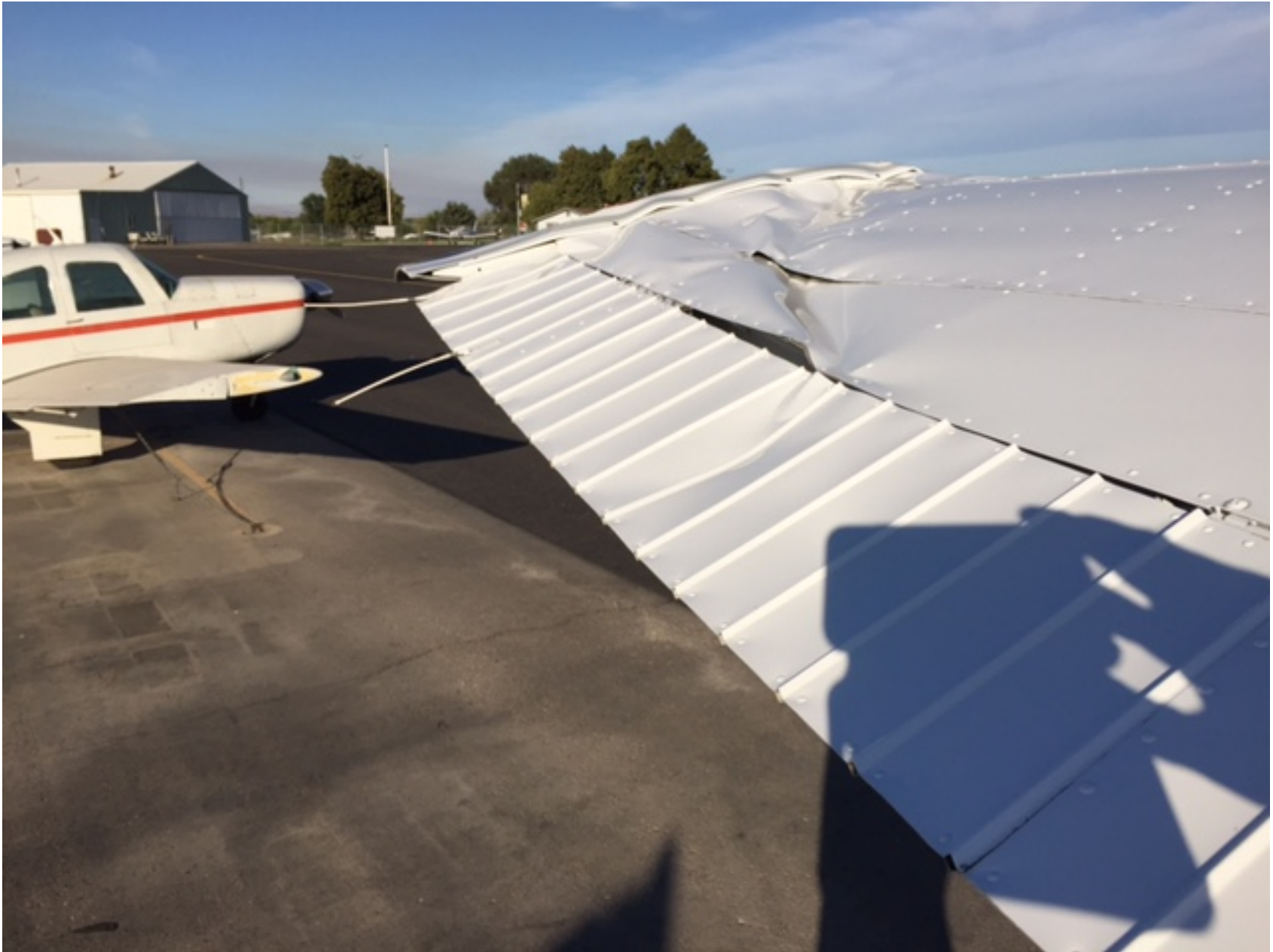
Photo 2 – Left Wing Damage (Photo Courtesy of FAA)
