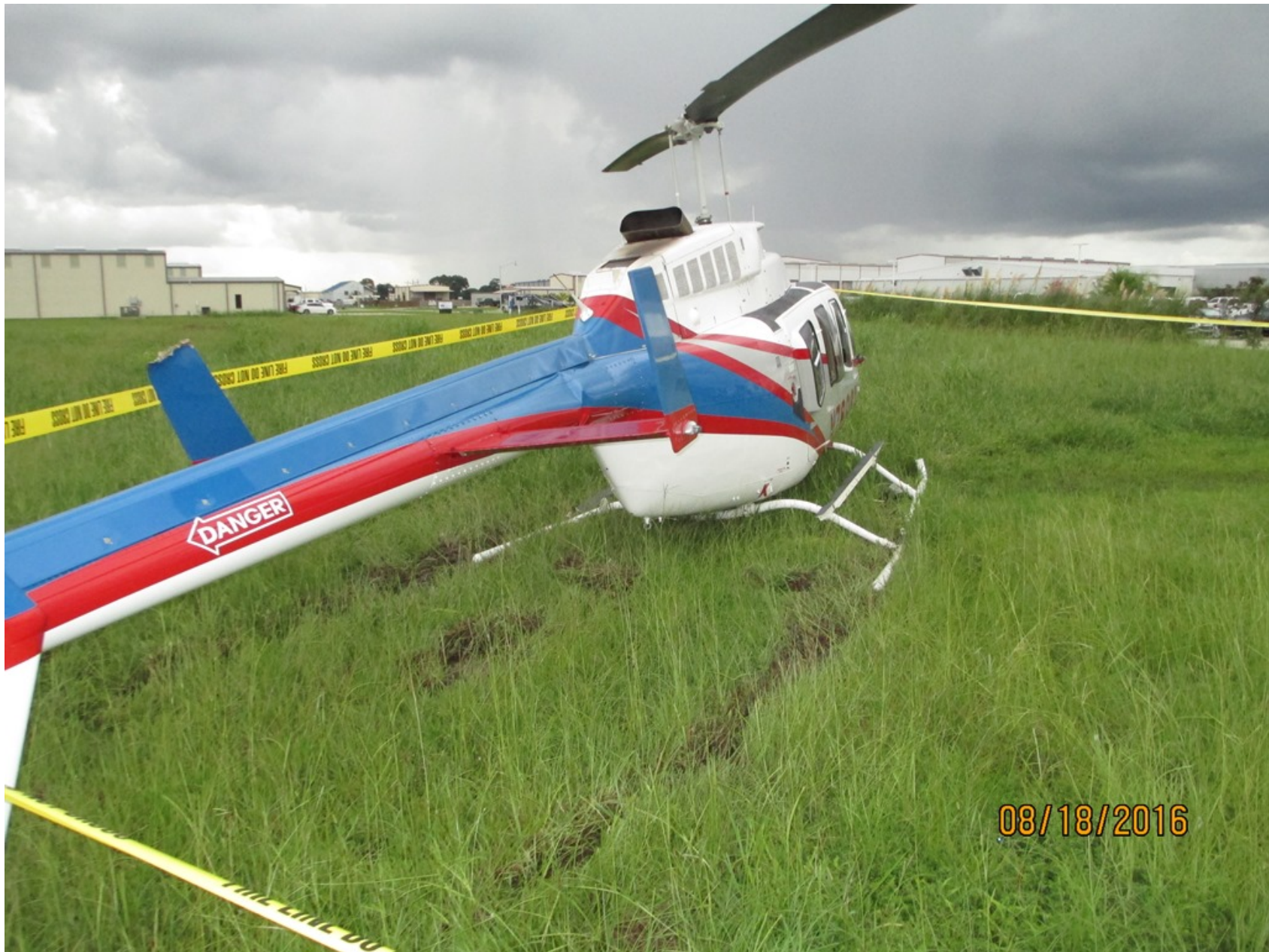
Photo 1 – View of damage to tailboom and vertical stabilizer (Courtesy of FAA)
