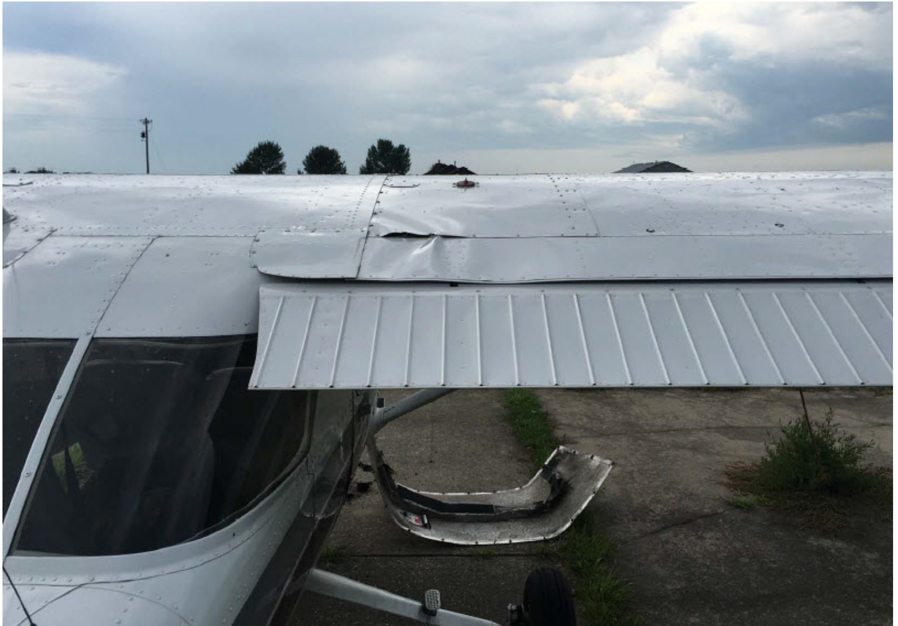
Photo 1 – View of the right wing damage (photo courtesy of the FAA)
