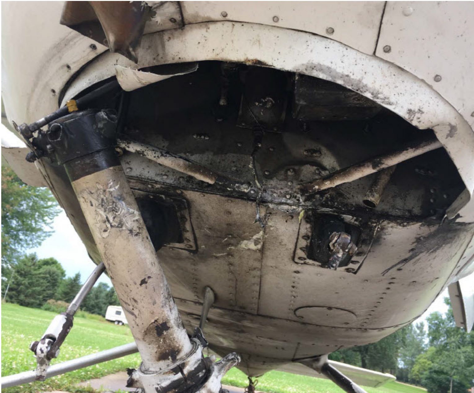
Photo 2 - View of the firewall damage (photo courtesy of the FAA)
