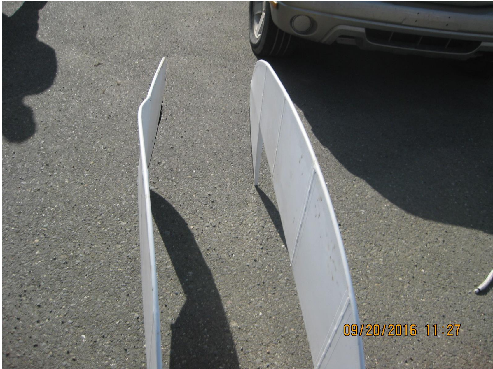
Photo 2 – View of damage to elevators (Photo courtesy of the FAA)
