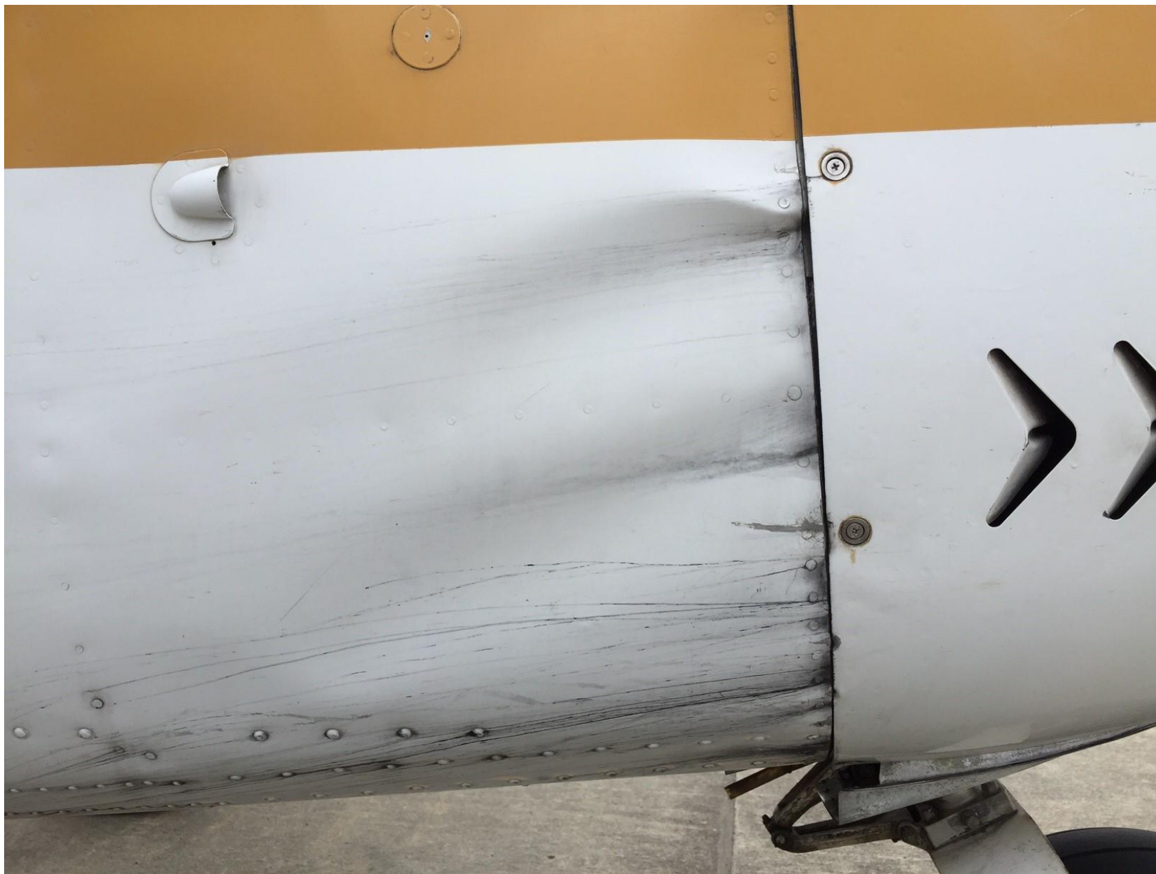
Photo 1 – View of substantial damage to the right side firewall of the airplane (Photo courtesy of the FAA)
