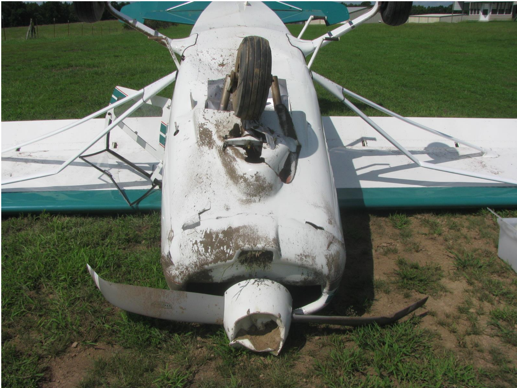
Photo 2 – View of damaged wing struts (photo courtesy of the FAA)
