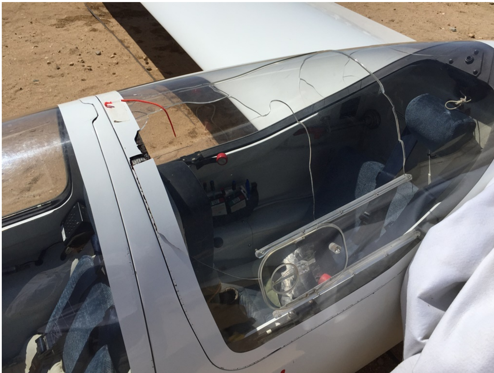
Photo 2 – View of damage to aft canopy (Courtesy of Operator)
