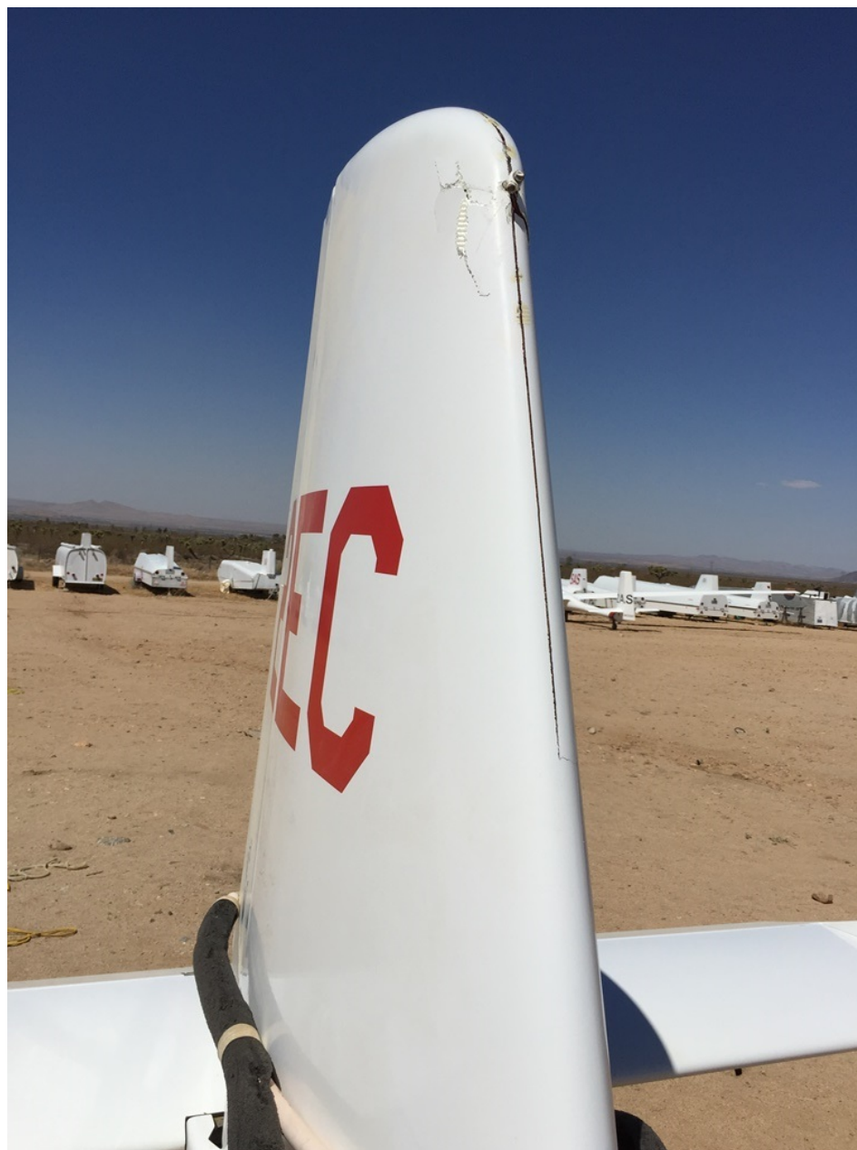
Photo 1 – View of damage to vertical stabilizer (Courtesy of Operator)
