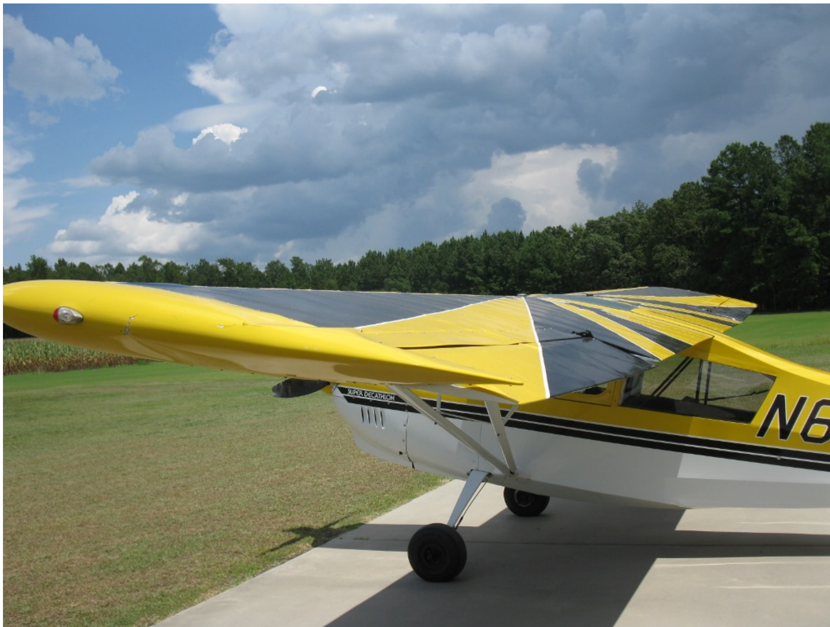
Photo 2 – View of damage to the left aileron (Courtesy of FAA)
