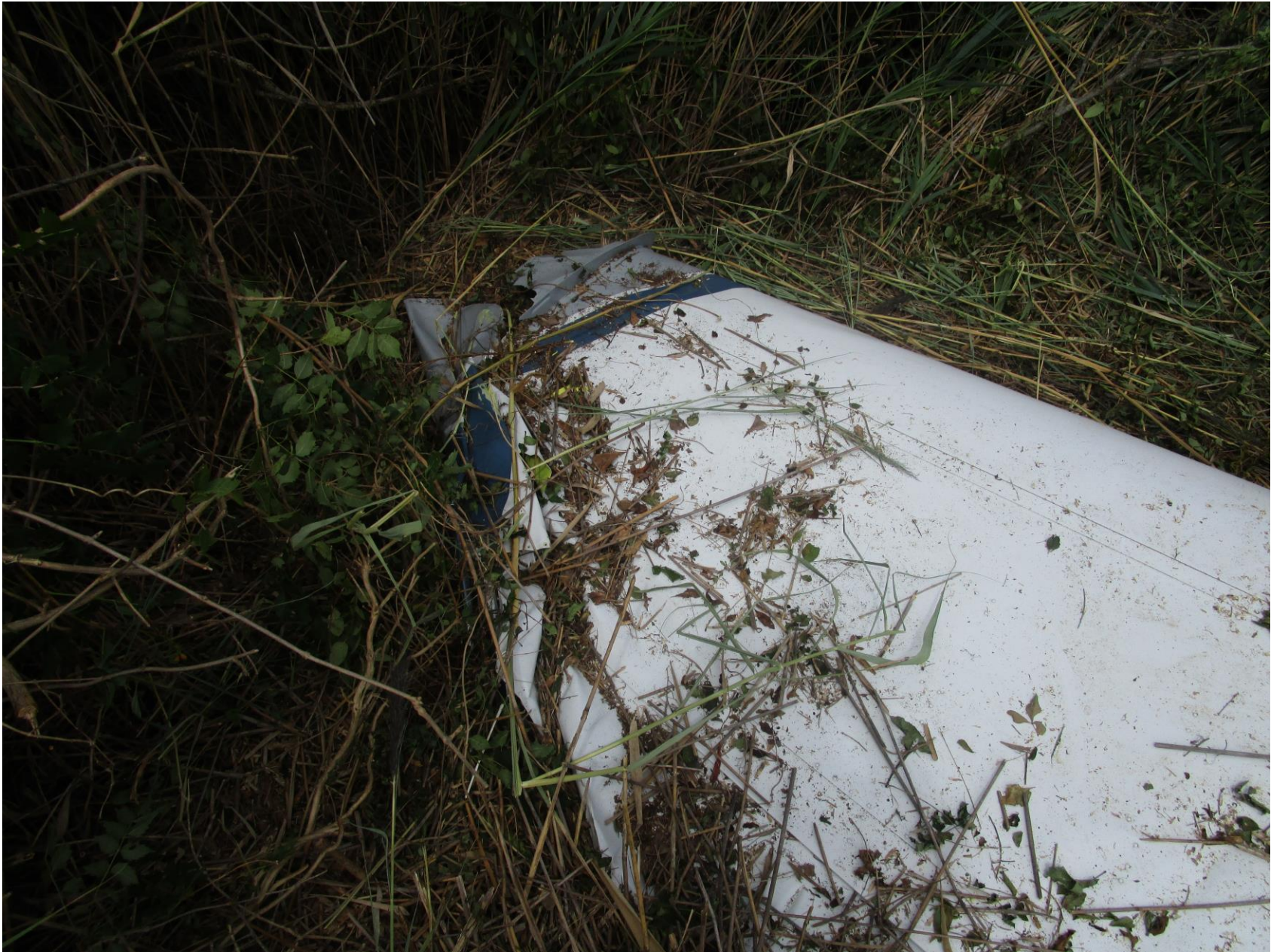
Photo 2 – Rear view of left wing and aileron damage (Photo courtesy of the FAA)
