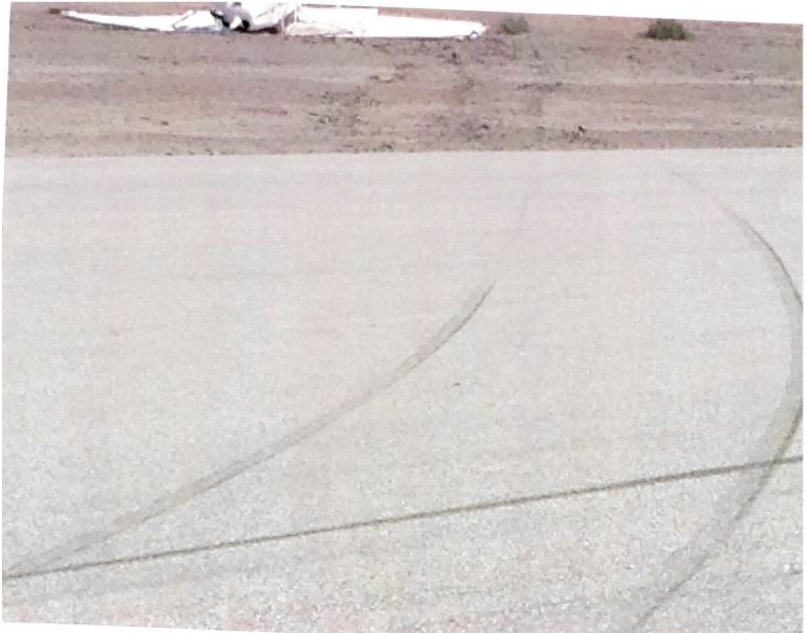
Photo 2 – Tire Marks Leading Off Runway (Photo Courtesy of FAA)
