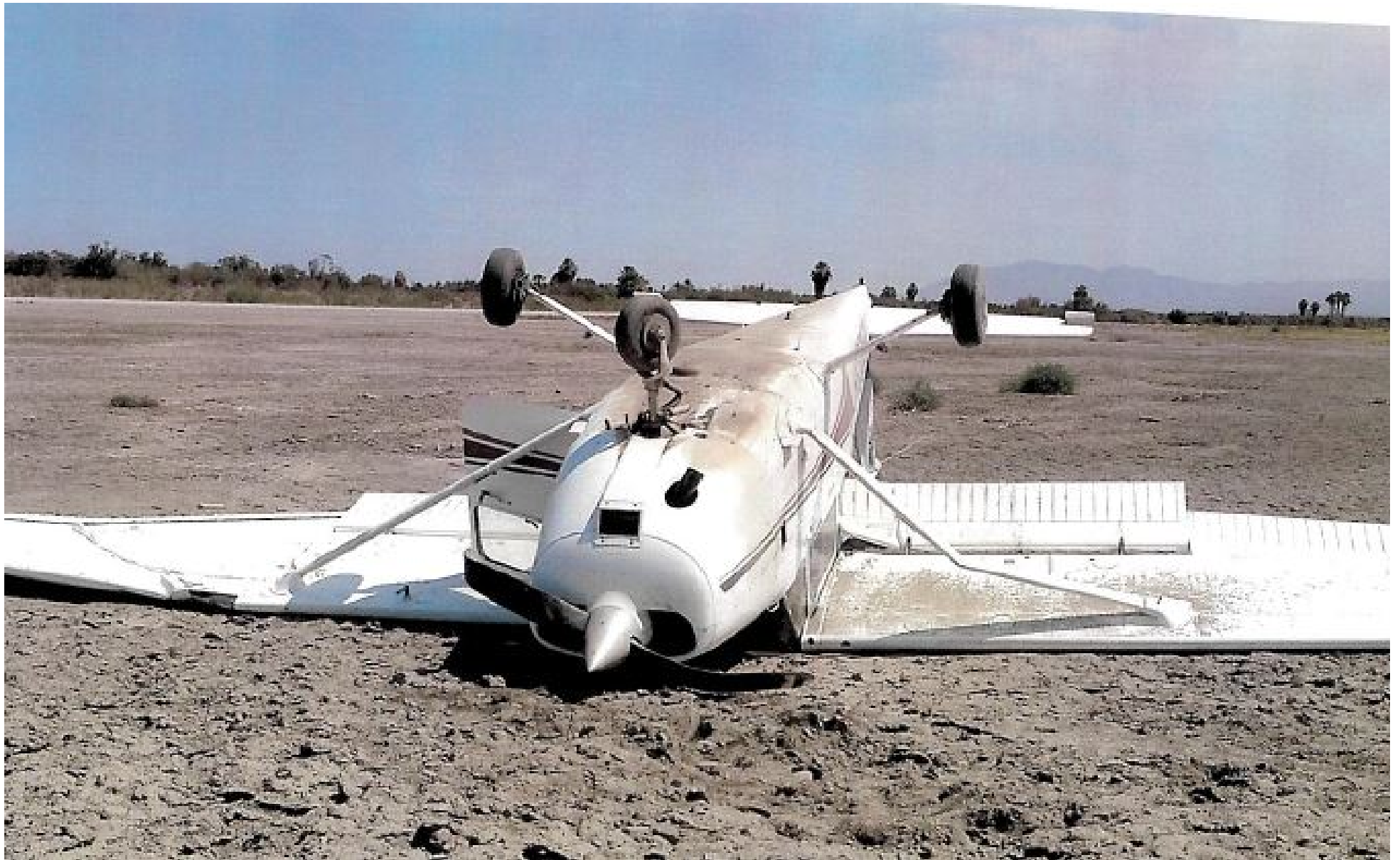
Photo 1 – Airplane Nosed Over (Photo Courtesy of FAA)
