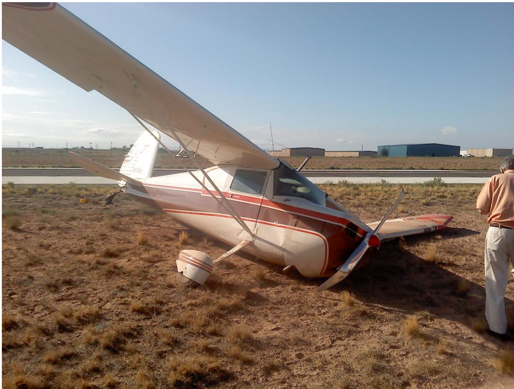
Photo 1 – Airplane off Runway with Substantially Damaged Left Wing (Photo Courtesy of FAA)
