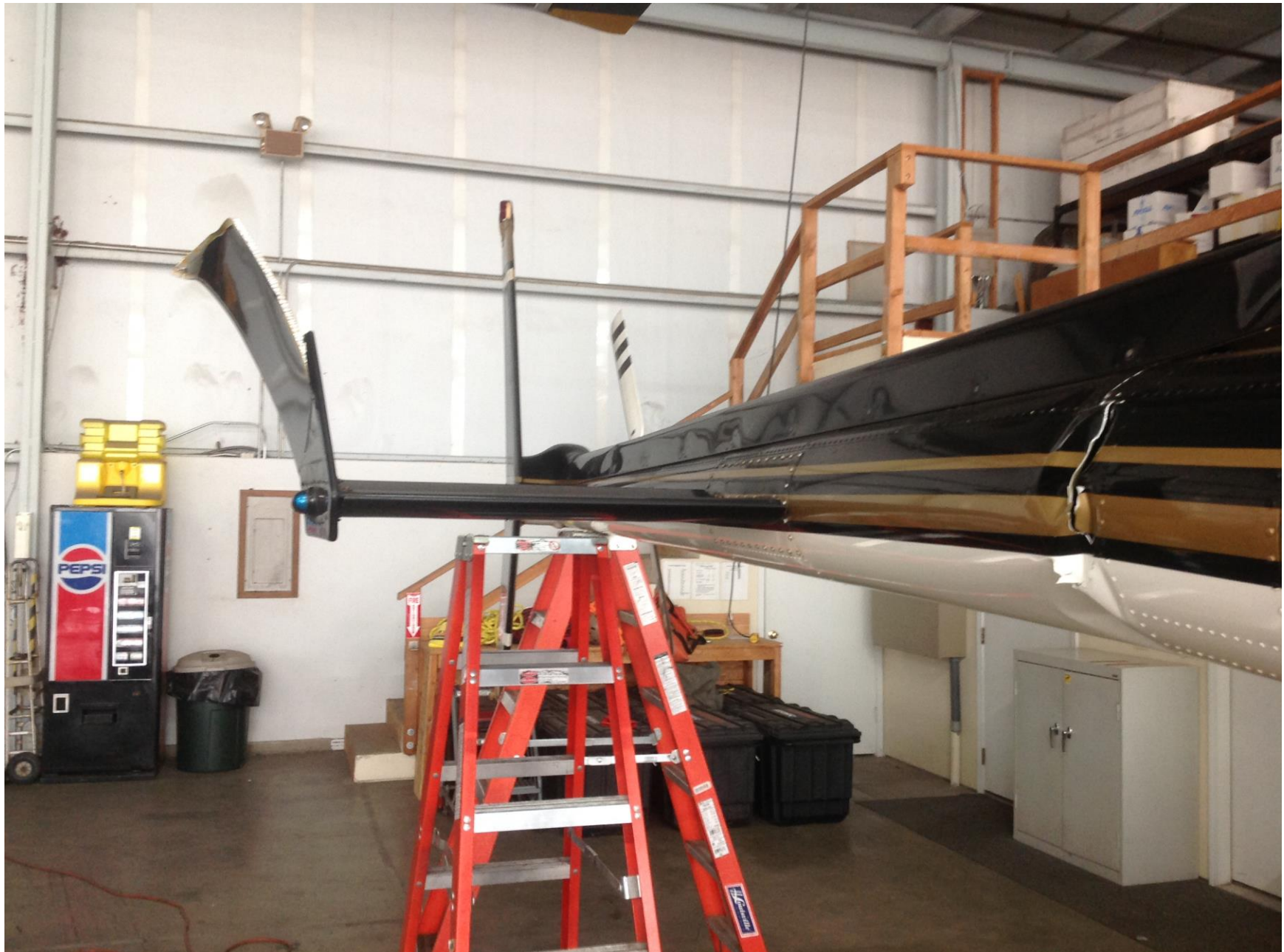
Photo 1 – View of tail boom damage (photo courtesy of the owner)
