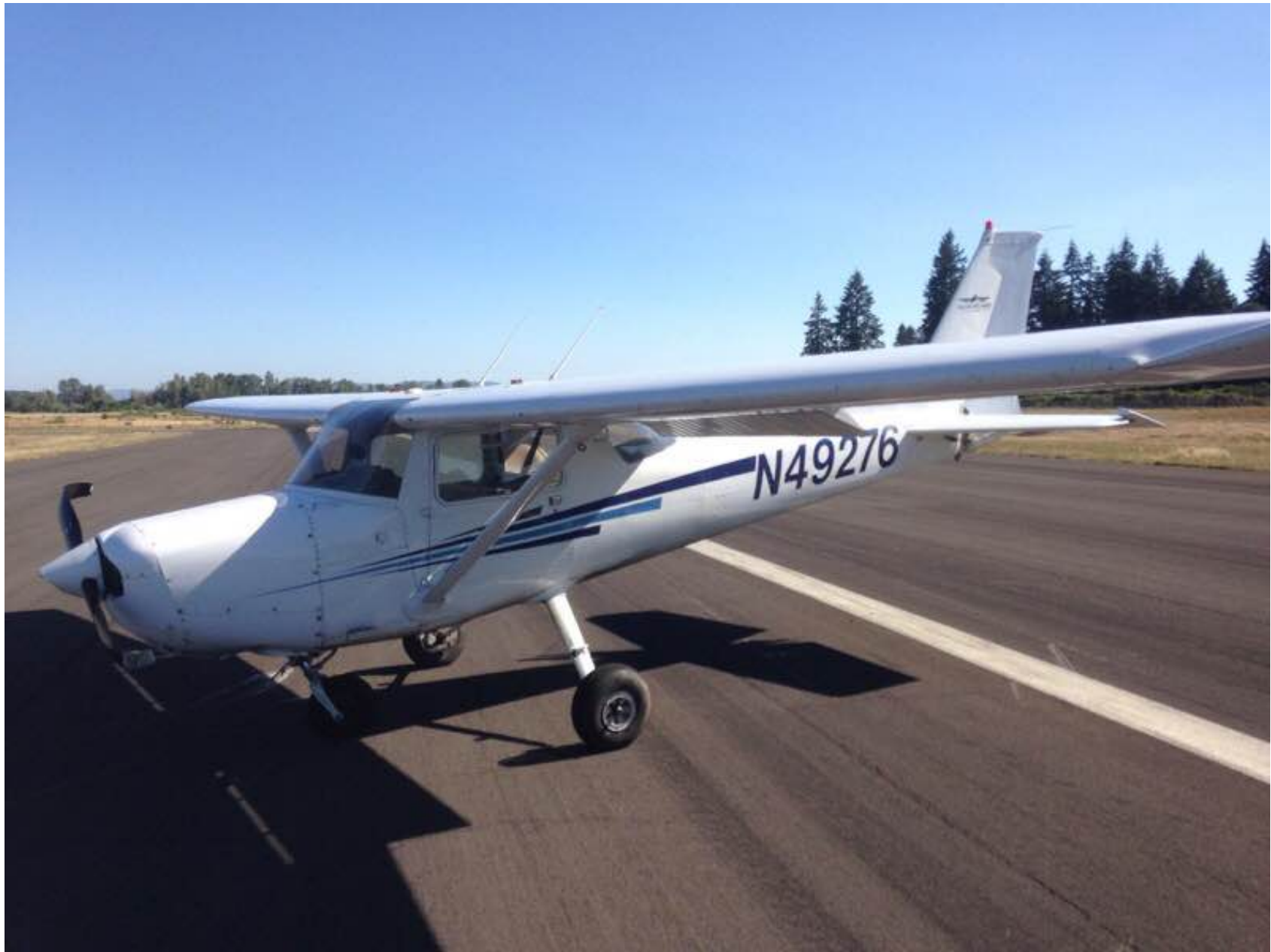
Photo 1 – Airplane with Partially Collapsed Nose Wheel (Photo Courtesy of Operator)
