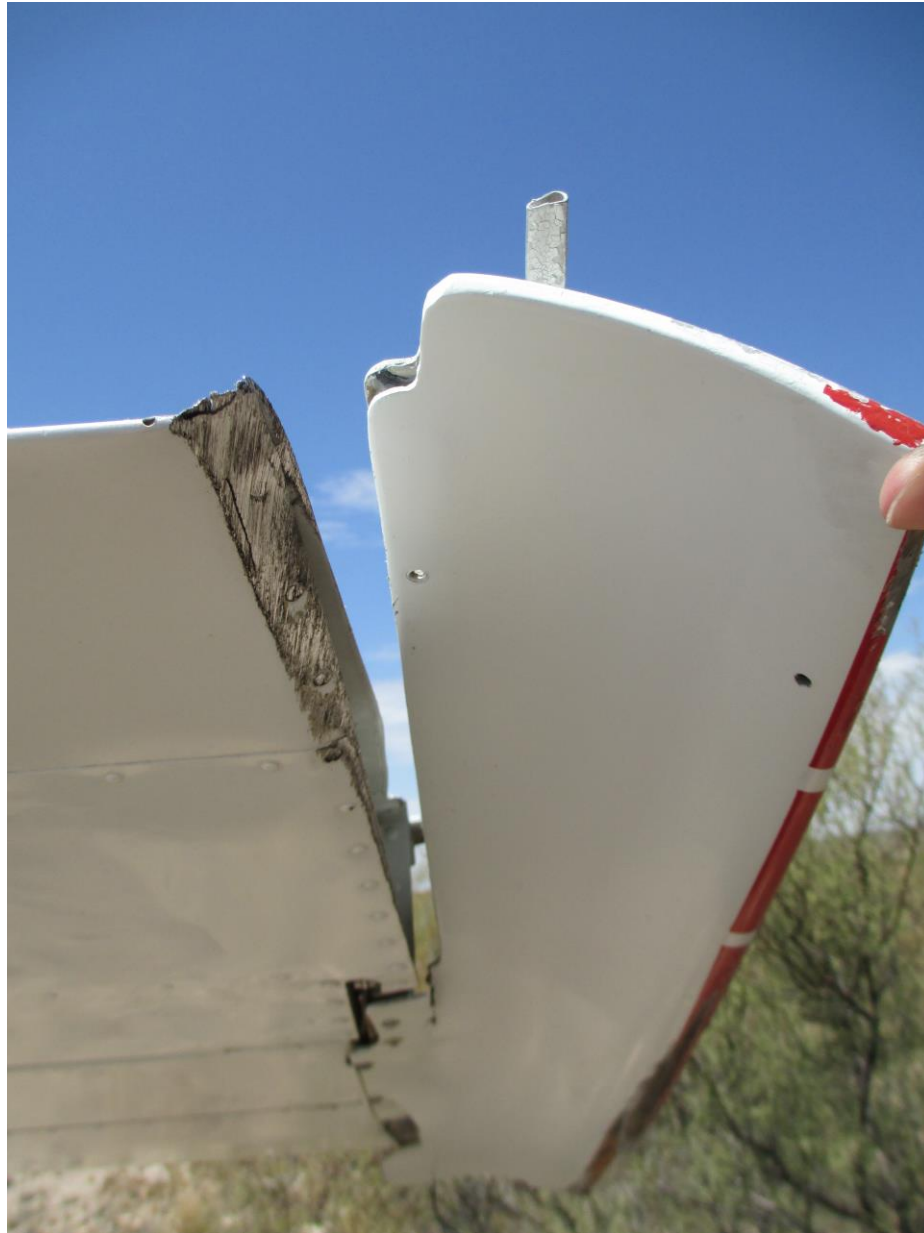
Photo 1 – View of right aileron damage (photo courtesy of the FAA)
