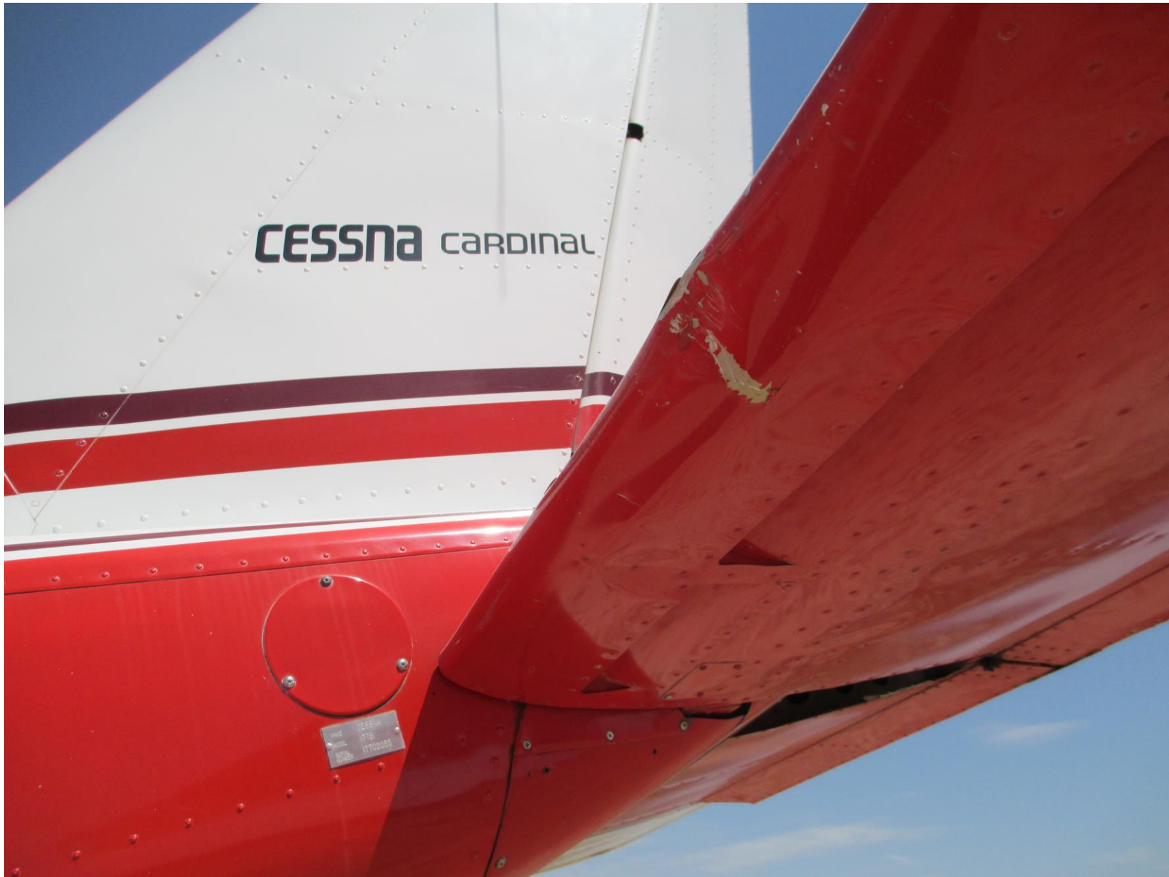
Photo 3 – View of empennage damage (photo courtesy of the FAA)
