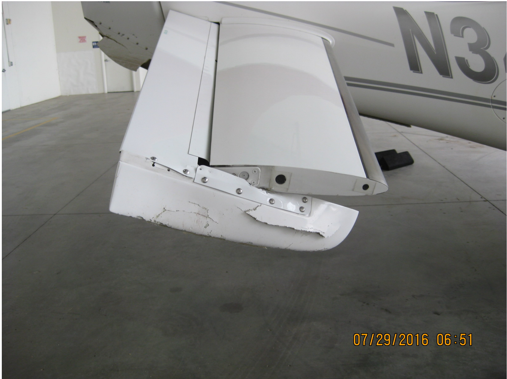
Photo 1 – Substantially Damaged Right Elevator (Photo Courtesy of FAA)
