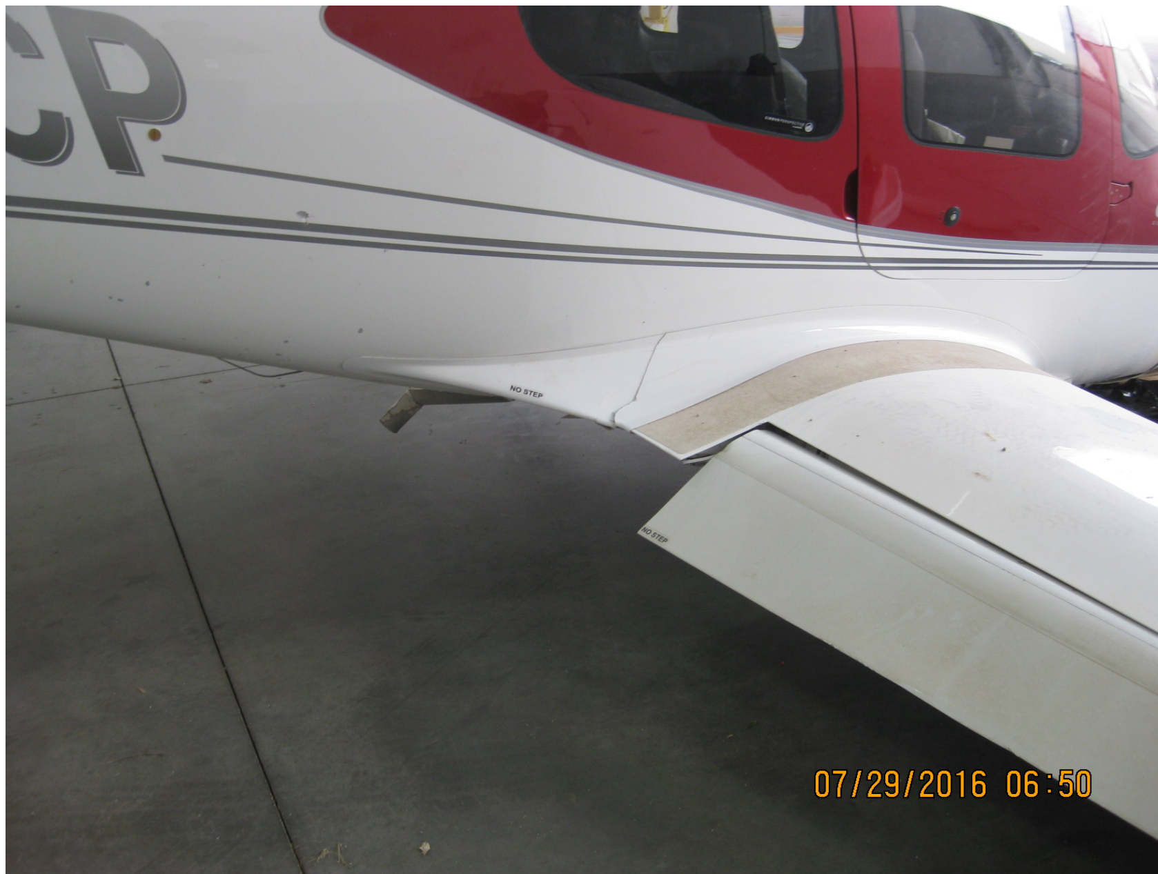
Photo 2 – Crack Visible on Substantially Damaged Right Wing (Photo Courtesy of FAA)
