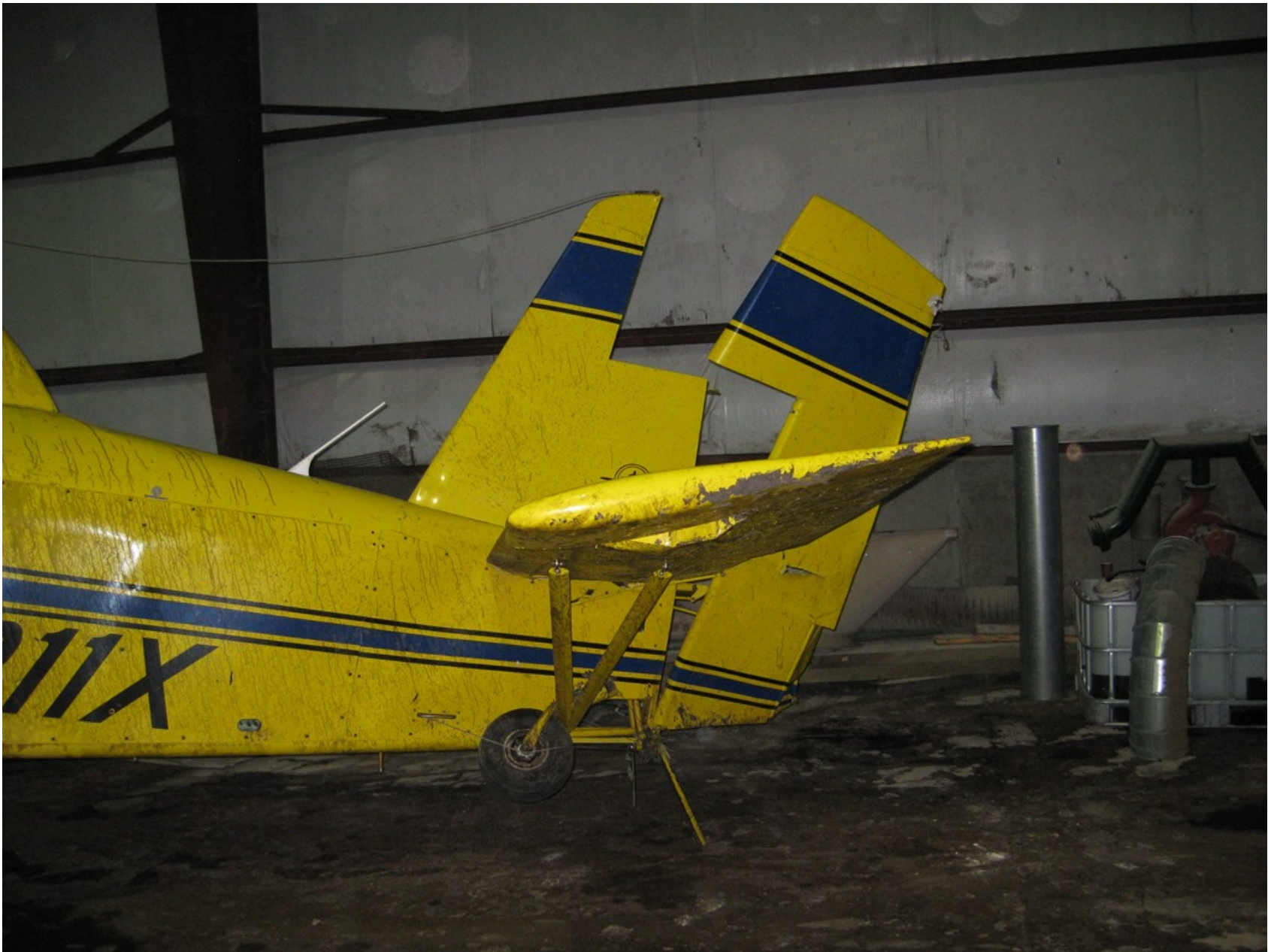
Photo 2 – View of damage to horizontal stabilizer and rudder (Courtesy of FAA)
