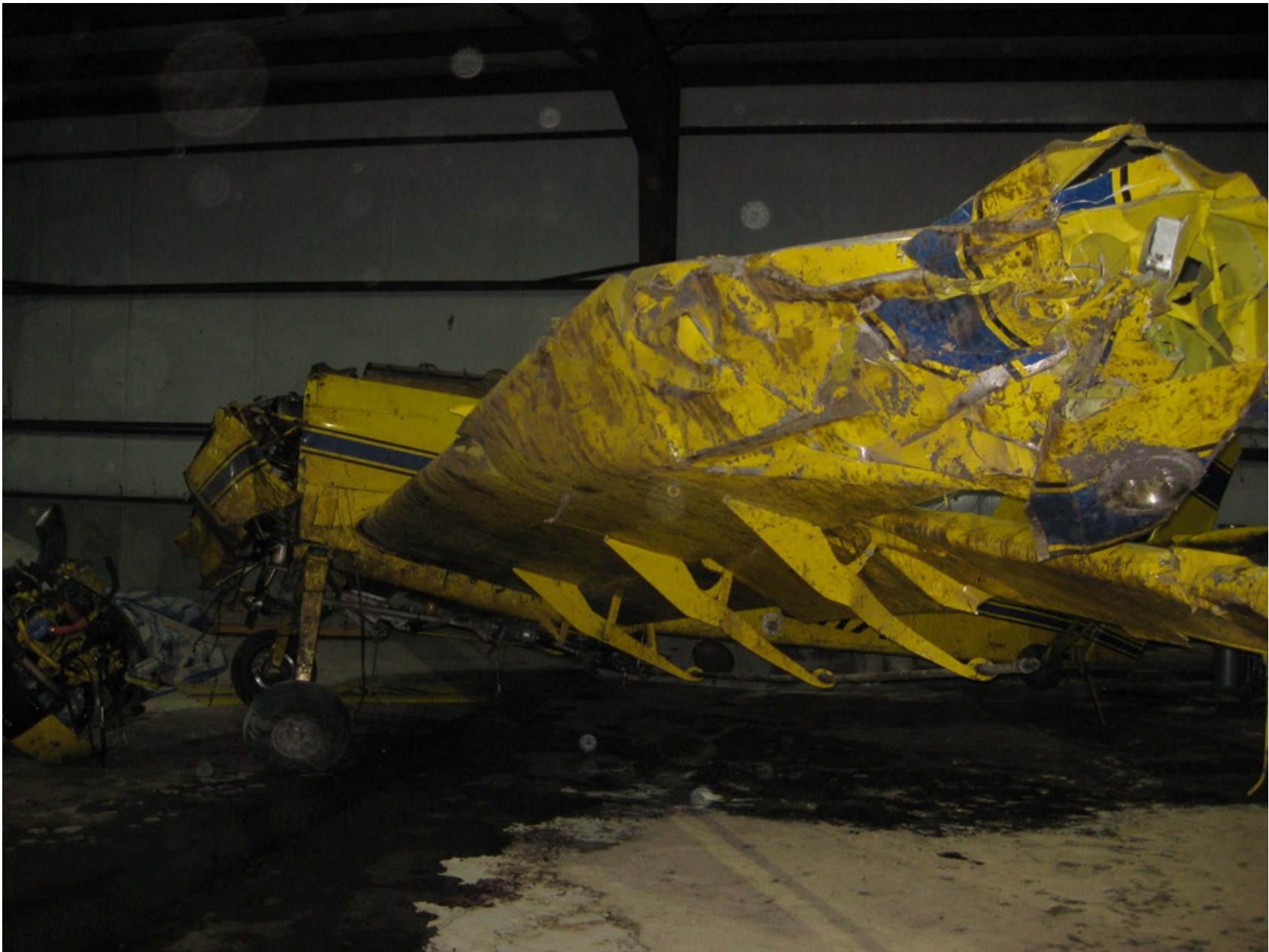
Photo 1 – View of damage to left wing spar, ribs and aileron (Courtesy of FAA)
