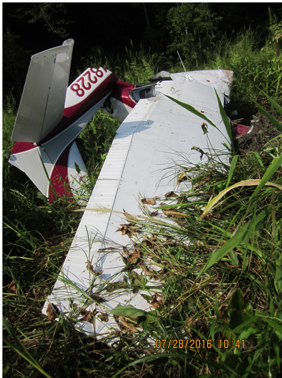
Photo 2 – Substantially Damaged Fuselage and Wings (Photo Courtesy of FAA)
