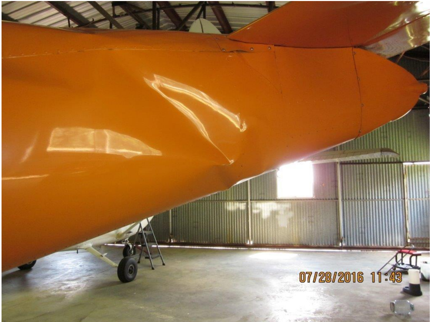
Photo 2 – Damage to left rear side of fuselage (Photo courtesy of the FAA)
