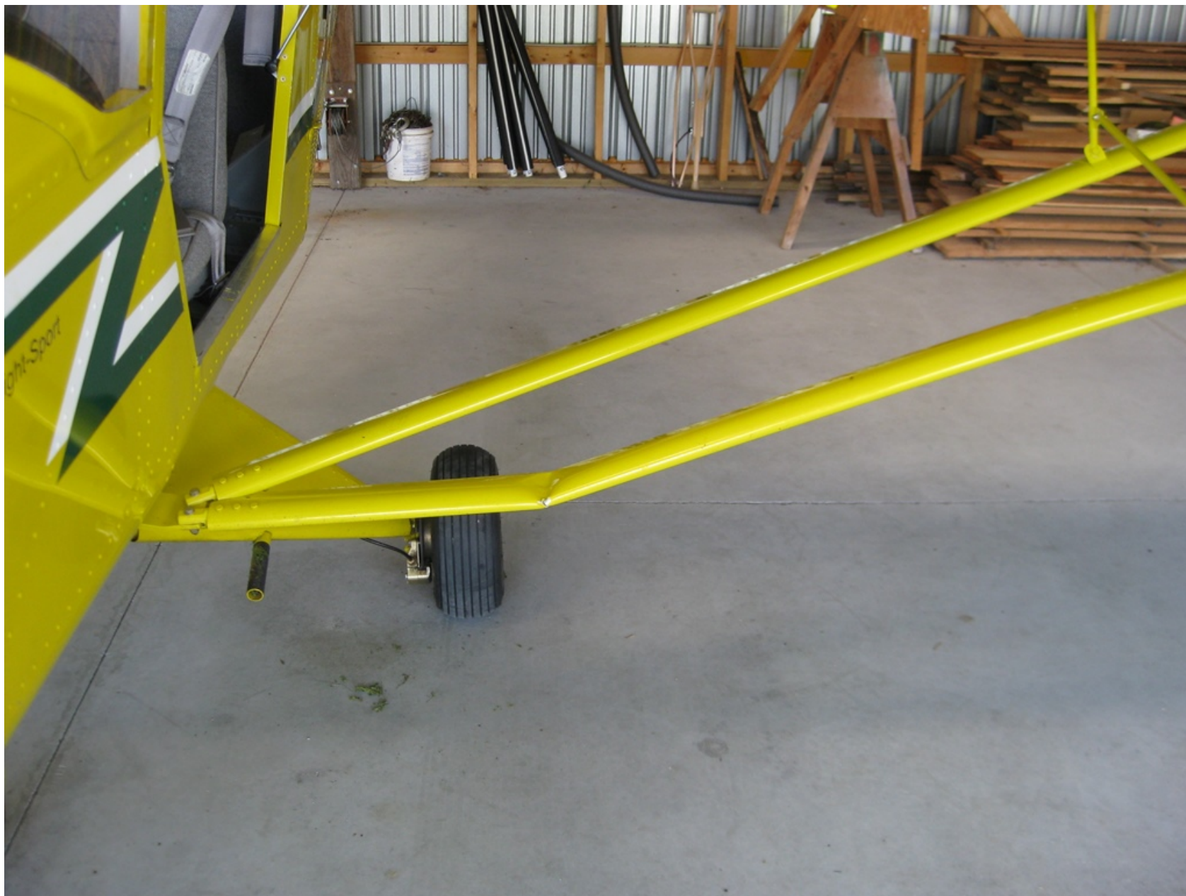
Photo 2 – View of damage to left wing strut (Courtesy of FAA)
