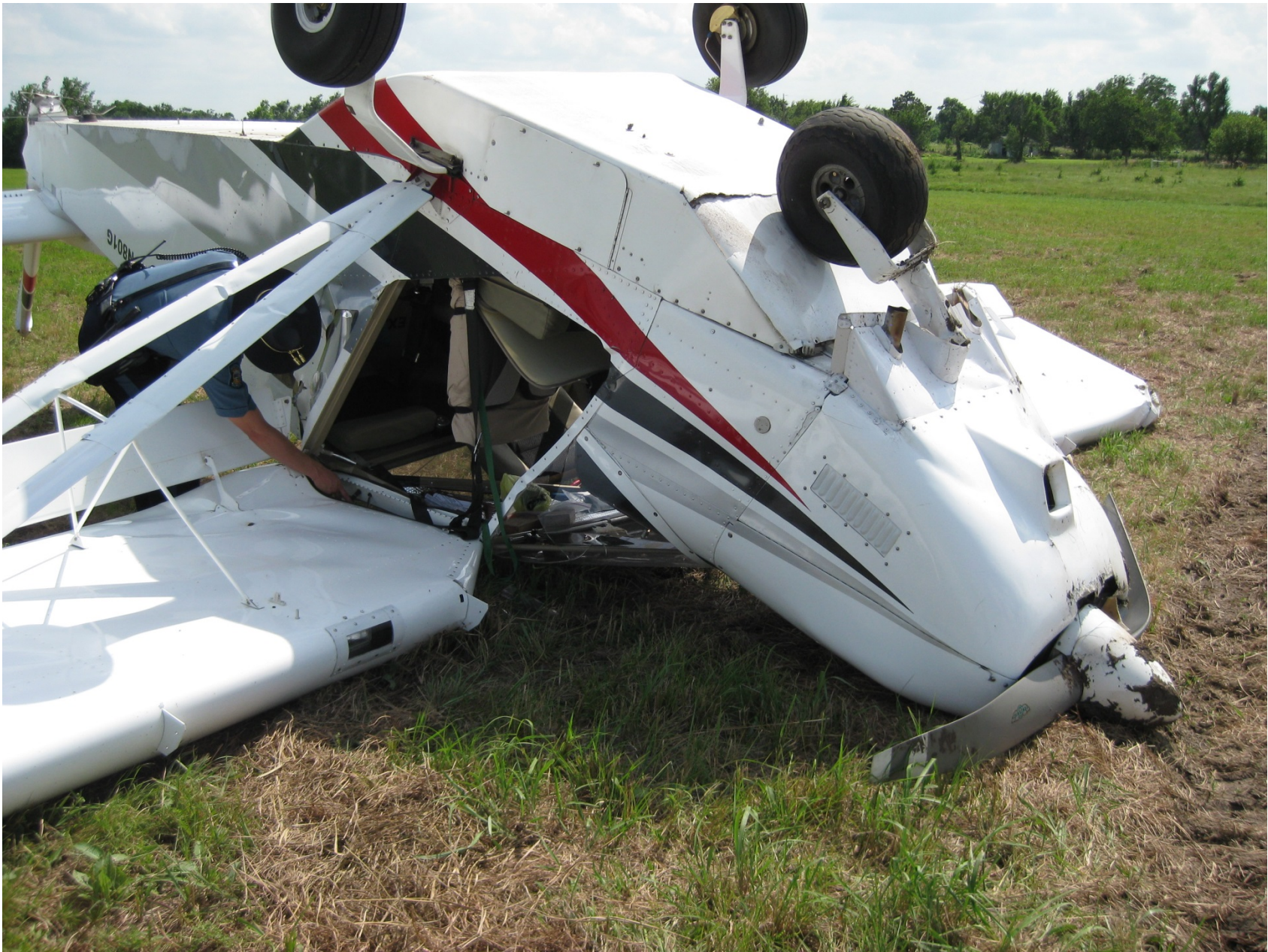
Photo 1 – Airplane Nosed Over (Photo Courtesy of FAA)
