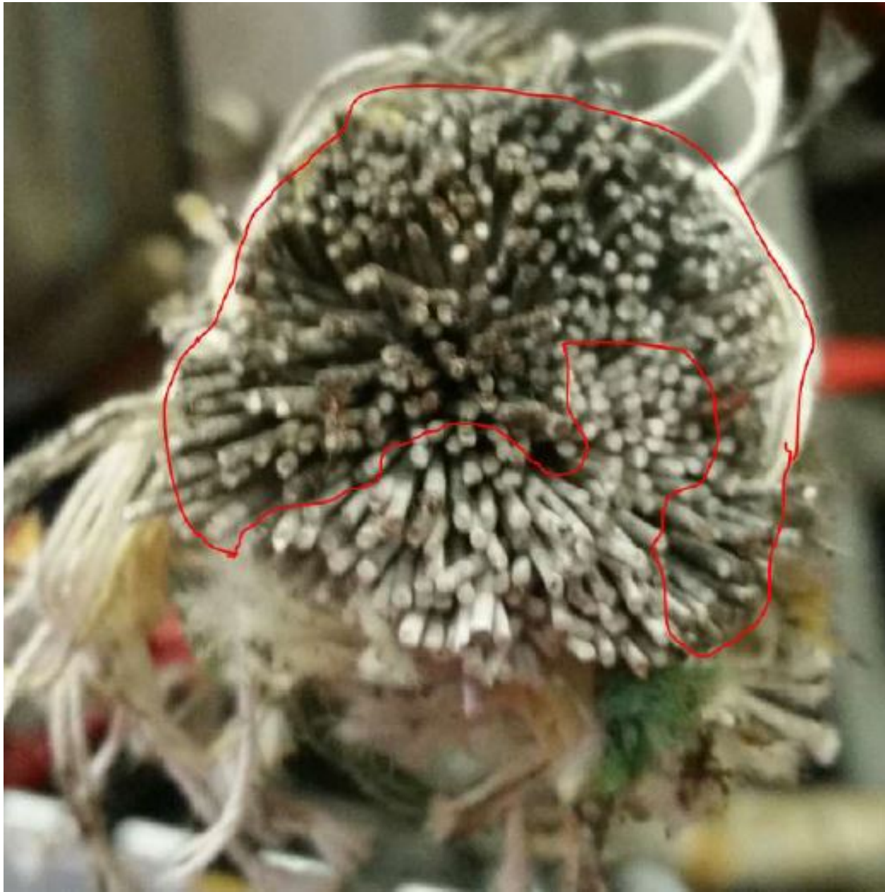
Photo 3 – Oil Residue on Nose Landing Gear Bungee (Photo Courtesy of Operator)
