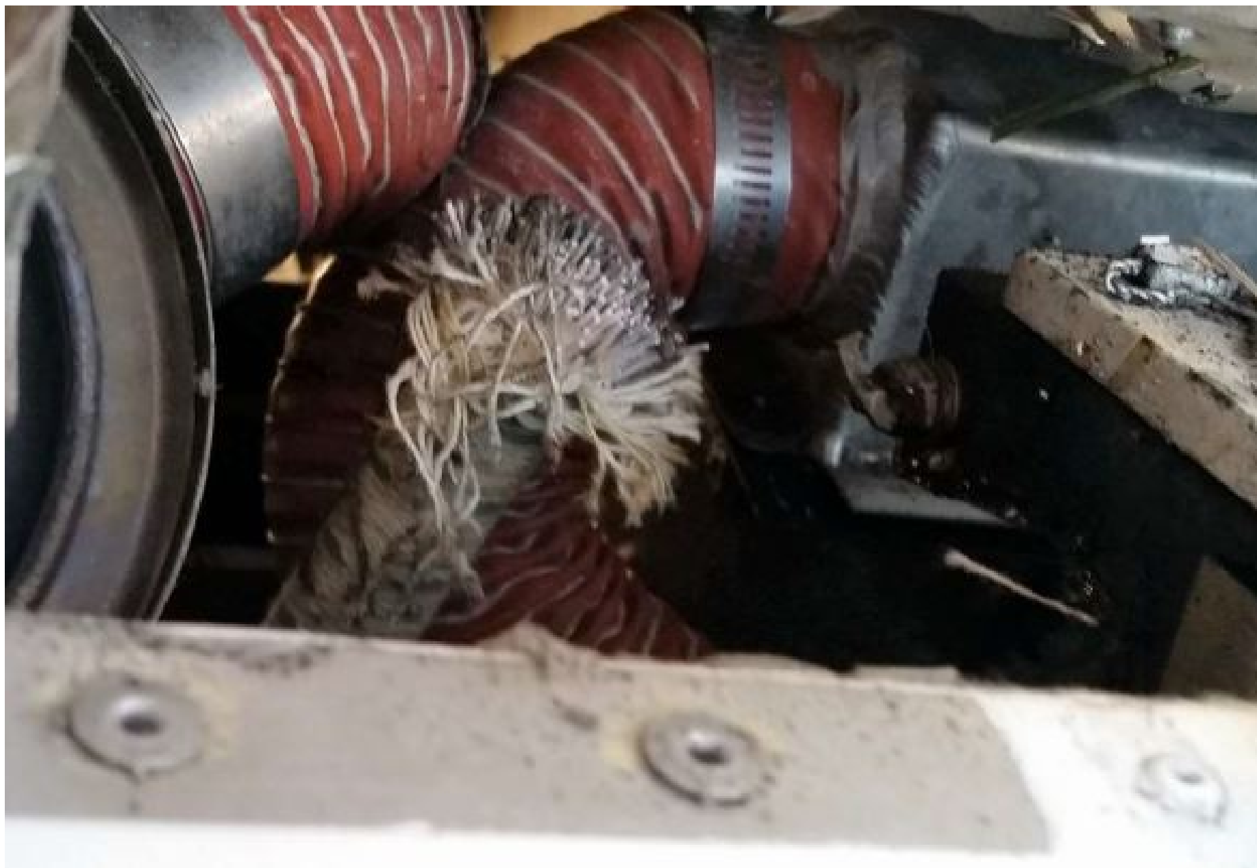
Photo 2 – Failed Nose Landing Gear Bungee (Photo Courtesy of Operator)
