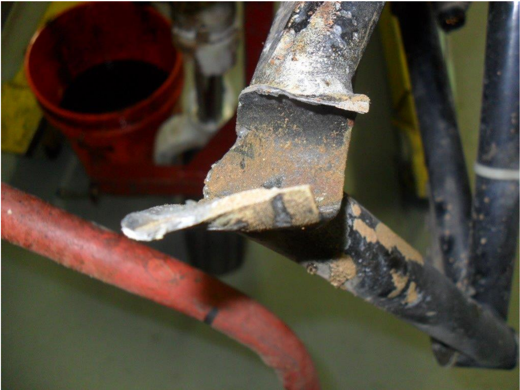
Photo 4 – View of damage to engine mount (Courtesy of FAA)
