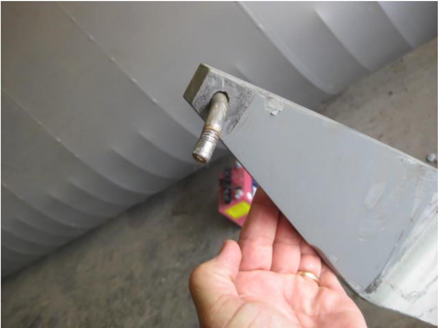
Photo 4 – Left landing gear attach bolt (Courtesy of the mechanic)
