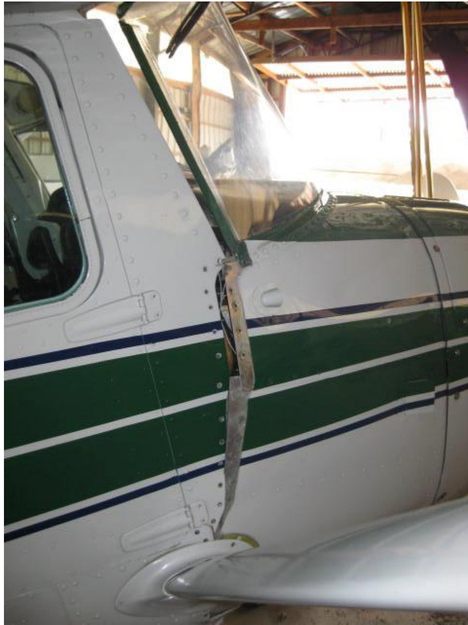
Photo 1 –View of right side fuselage separation (Courtesy of the FAA)
