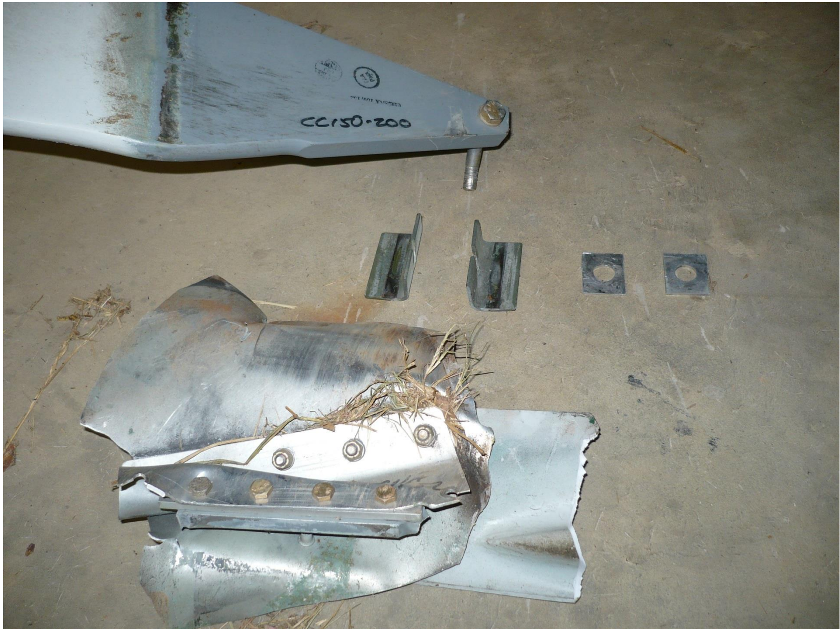
Photo 5 – Torn left landing gear support and gear leg (Courtesy of the mechanic)
