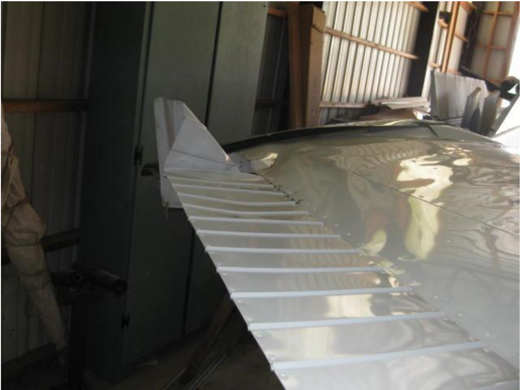
Photo 3 – Left wing trailing edge and aileron damage (Courtesy of the FAA)
