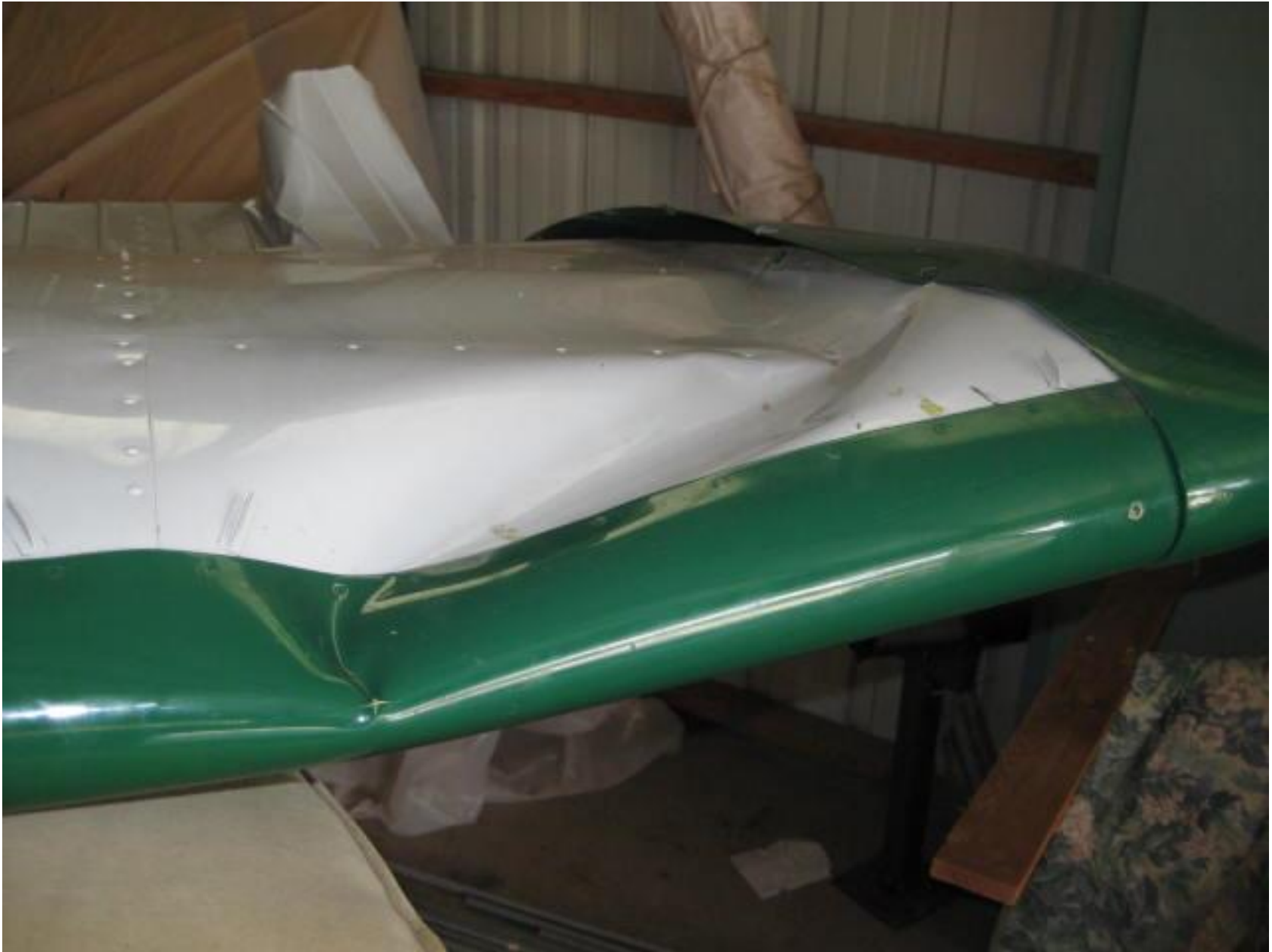
Photo 2 – Left wing leading edge damage (Courtesy of the FAA)
