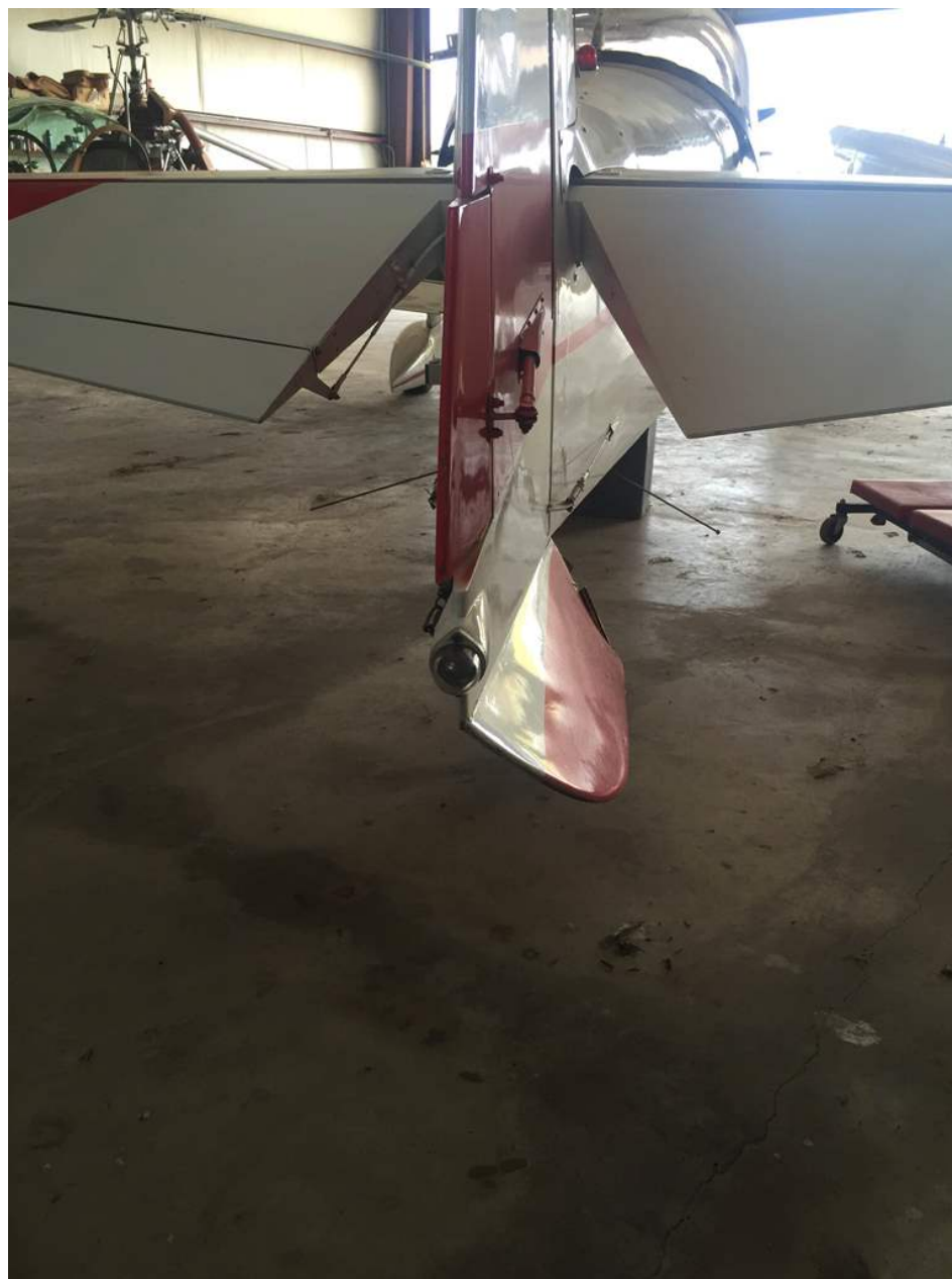
Photo 1 – View of damage to rudder (Courtesy of FAA)
