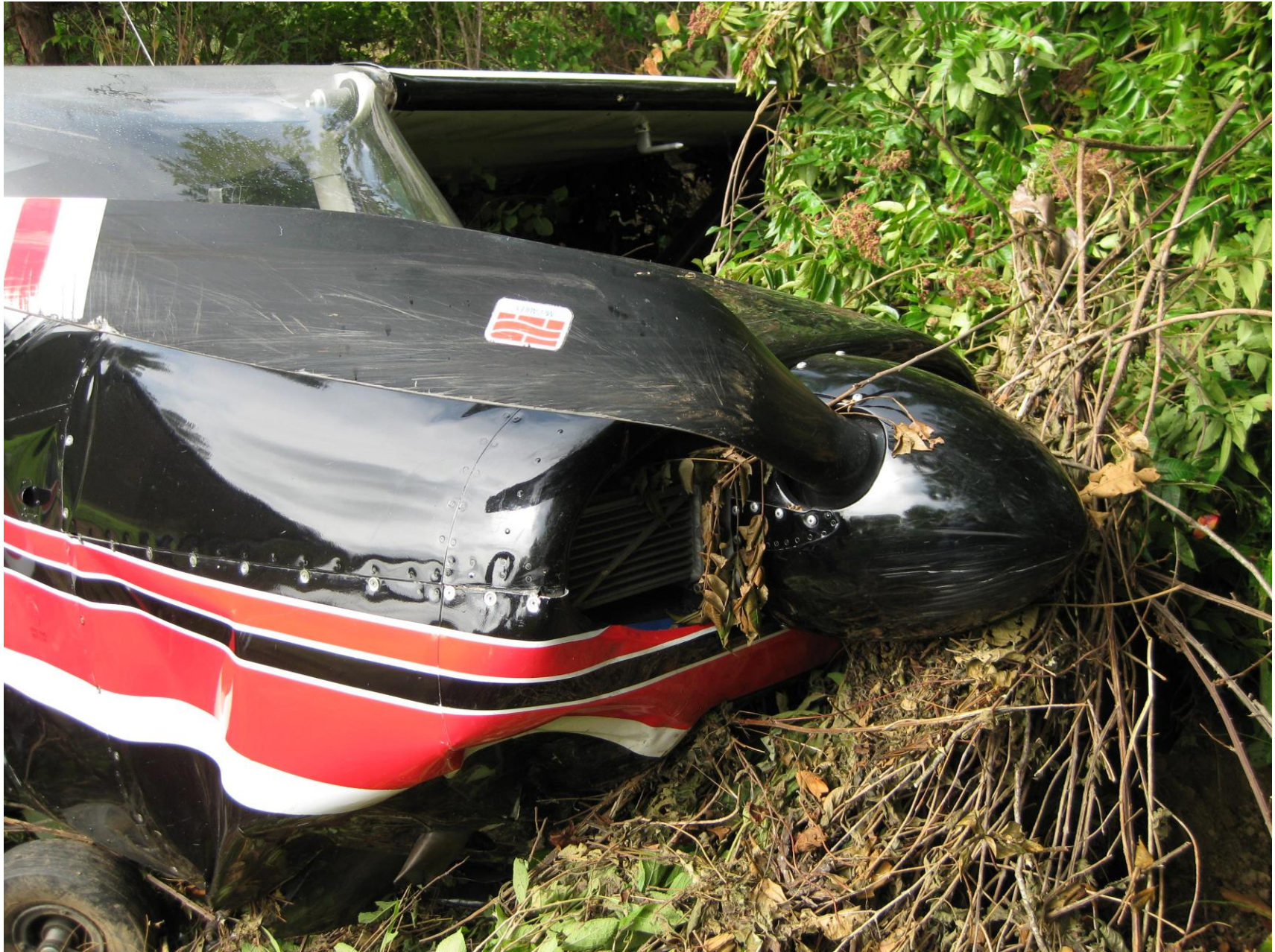
Photo 2 – View of substantial damage to the fuselage (photo courtesy of the FAA)
