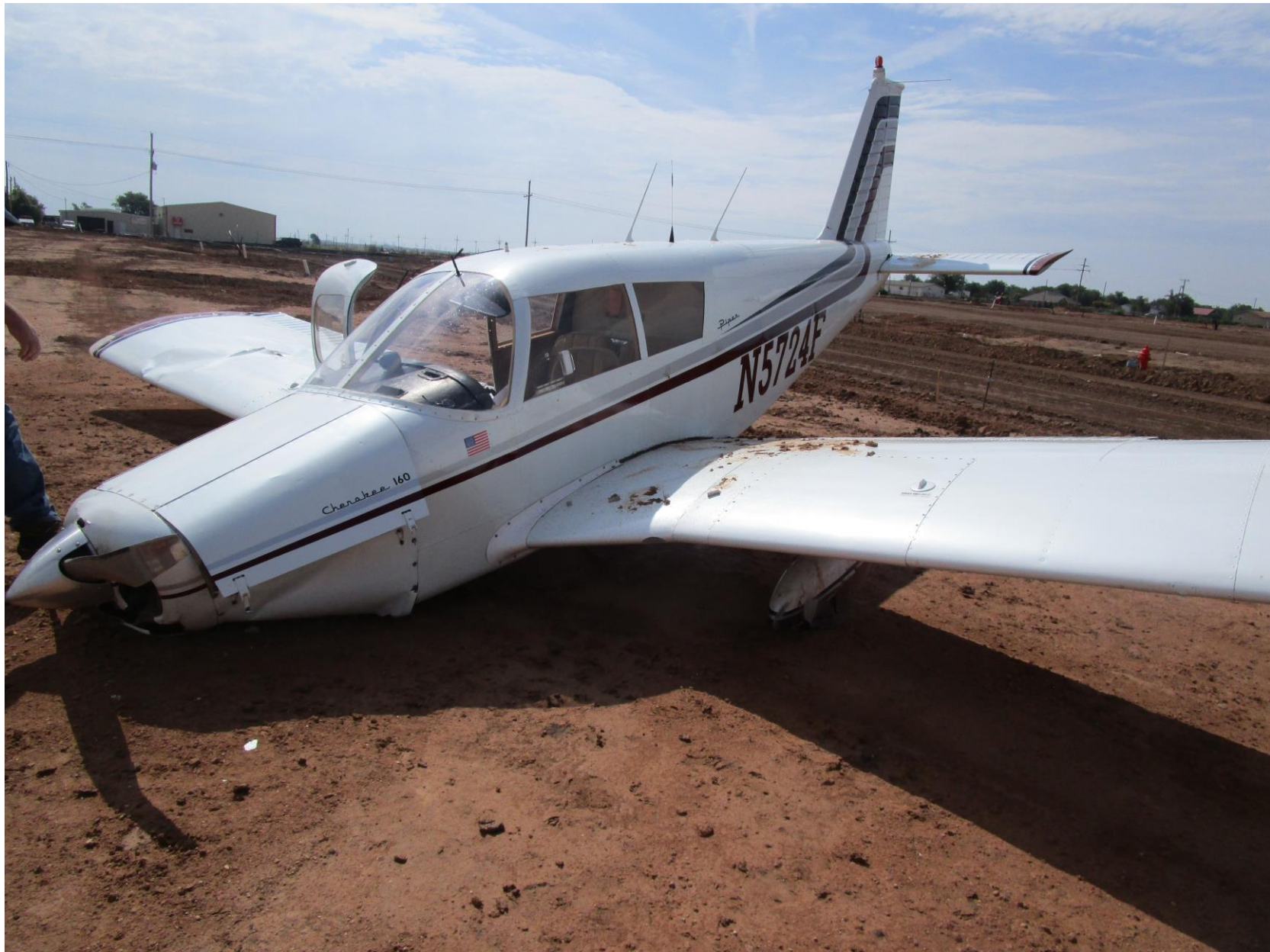
Photo 1 – View of substantial damage to the fuselage and right wing (photo courtesy of the FAA)
