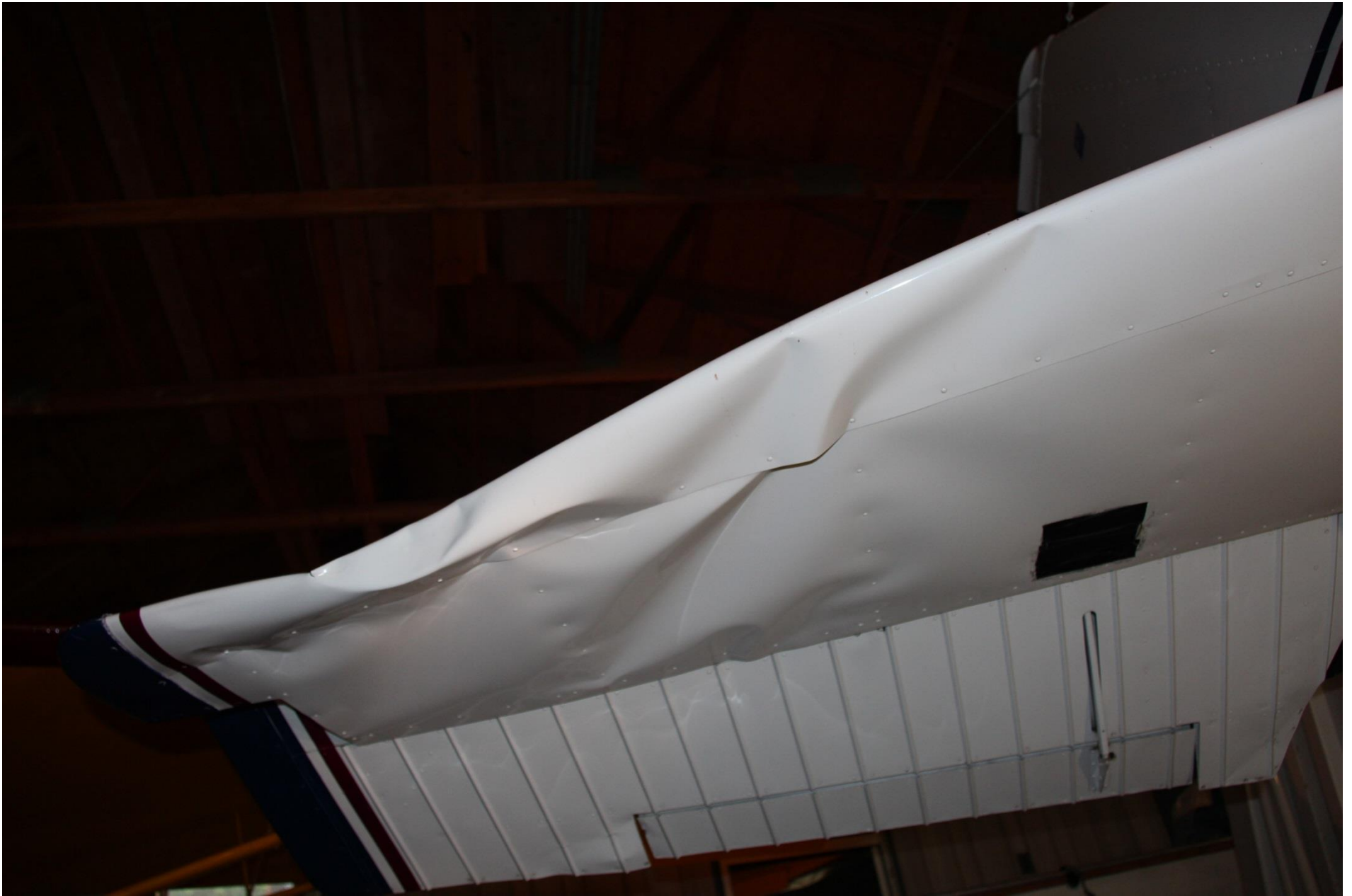
Photo 1 – Underside view of damaged right rear horizontal stabilizer and elevator (Courtesy of the FAA)
