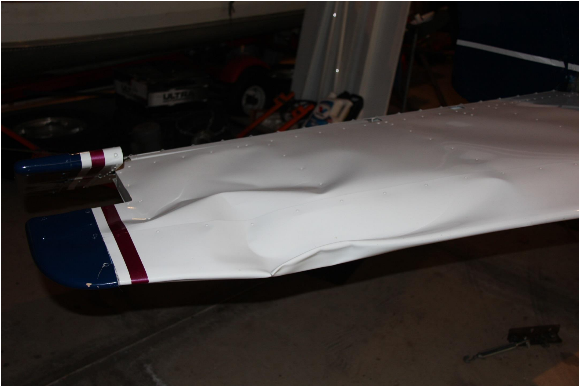
Photo 2 - Top view of damaged right rear horizontal stabilizer (Courtesy of the FAA)
