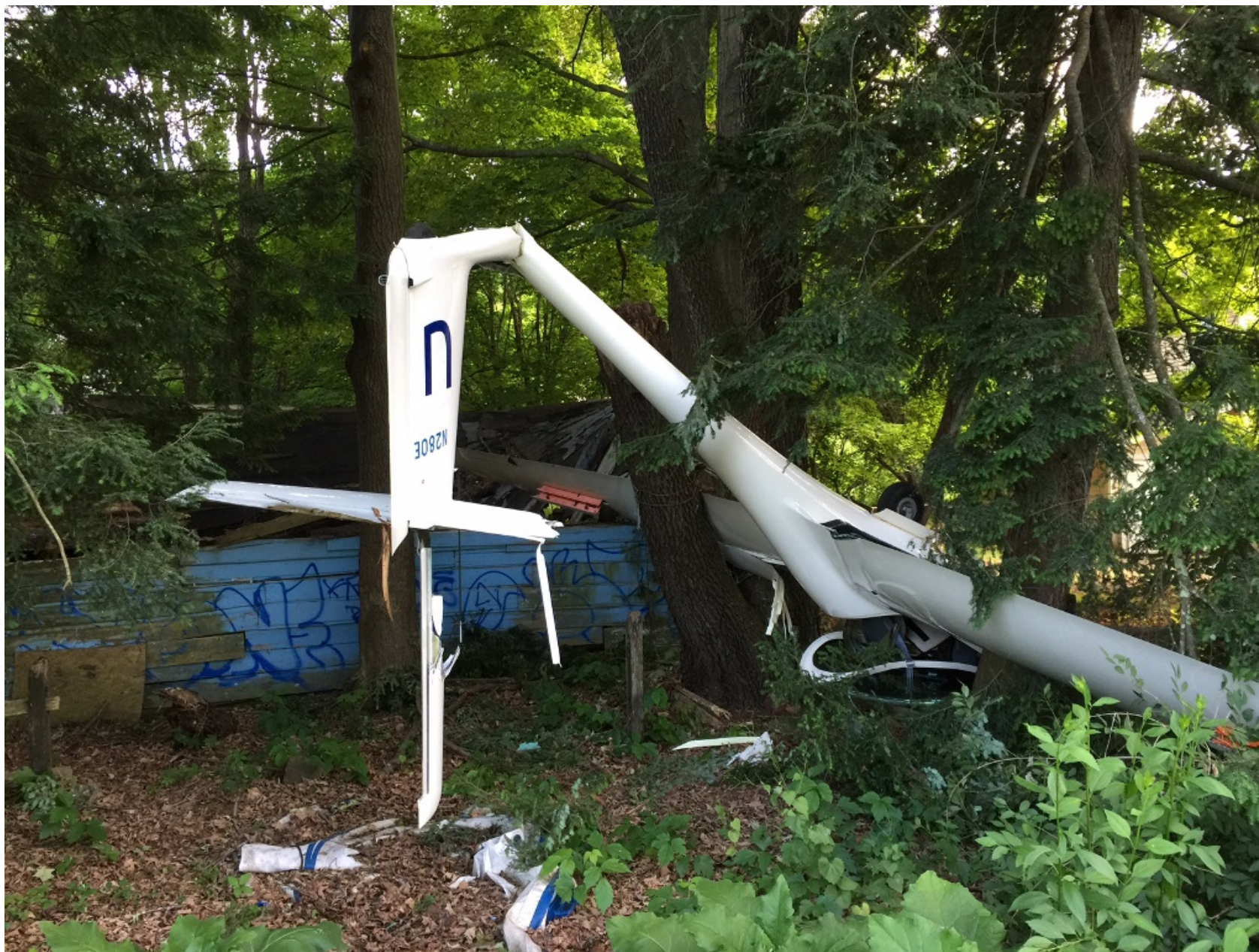
Photo 2 – View of damage to both wings and empennage (Courtesy of FAA)
