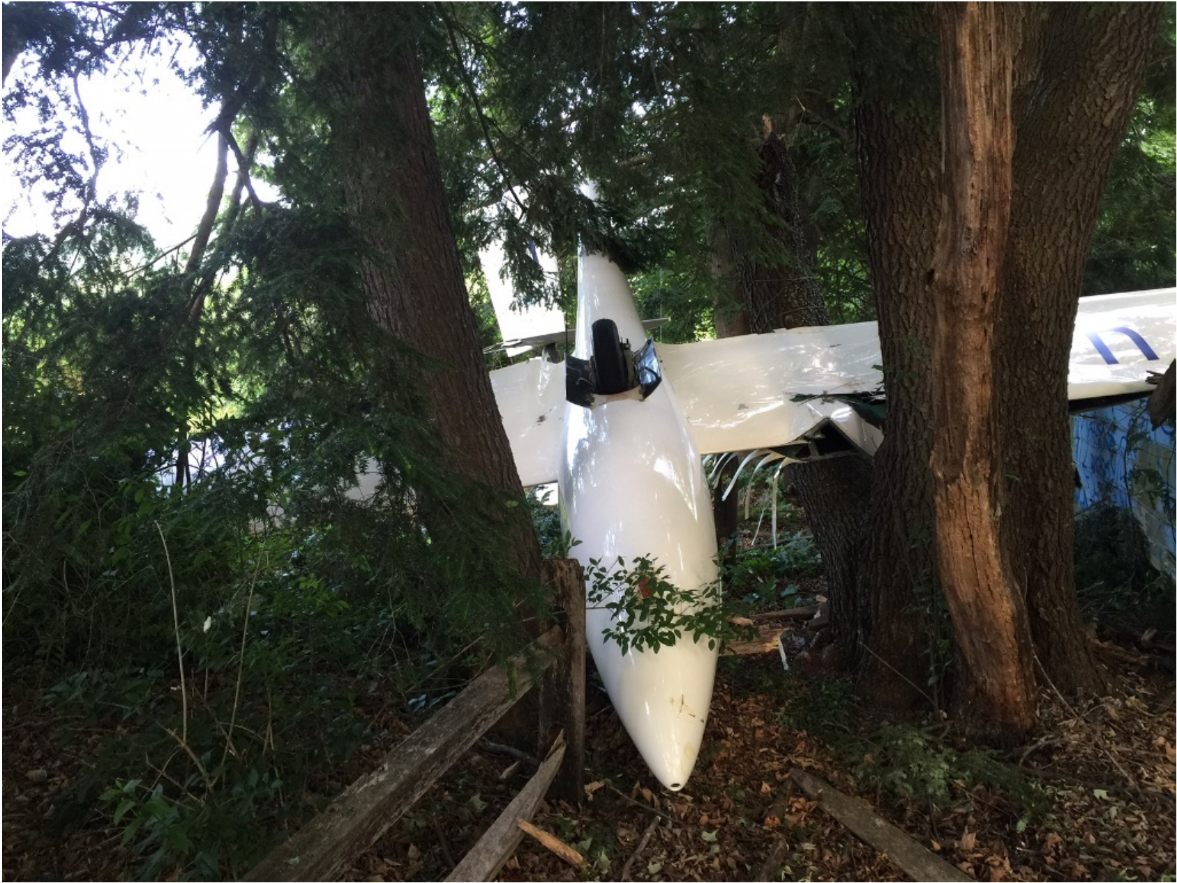
Photo 1 – View of inverted glider with damage to right wing and empennage (Courtesy of FAA)
