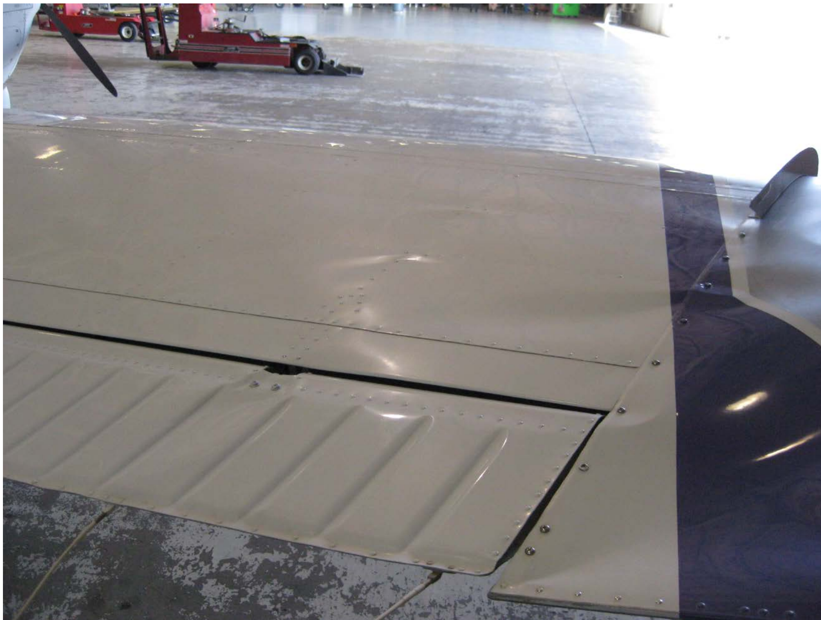
Photo 1 – View of right aileron damage (photo courtesy of the FAA)
