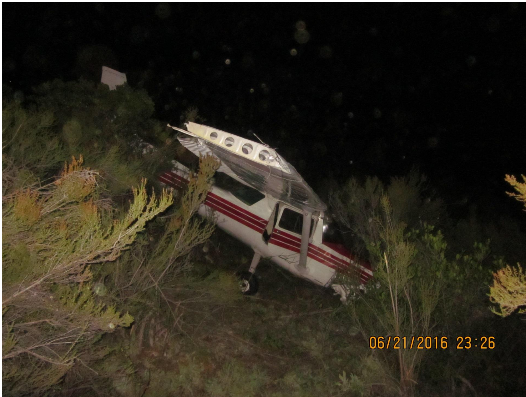
Photo 1 – View of fuselage and right aileron damage (photo courtesy of the FAA)
