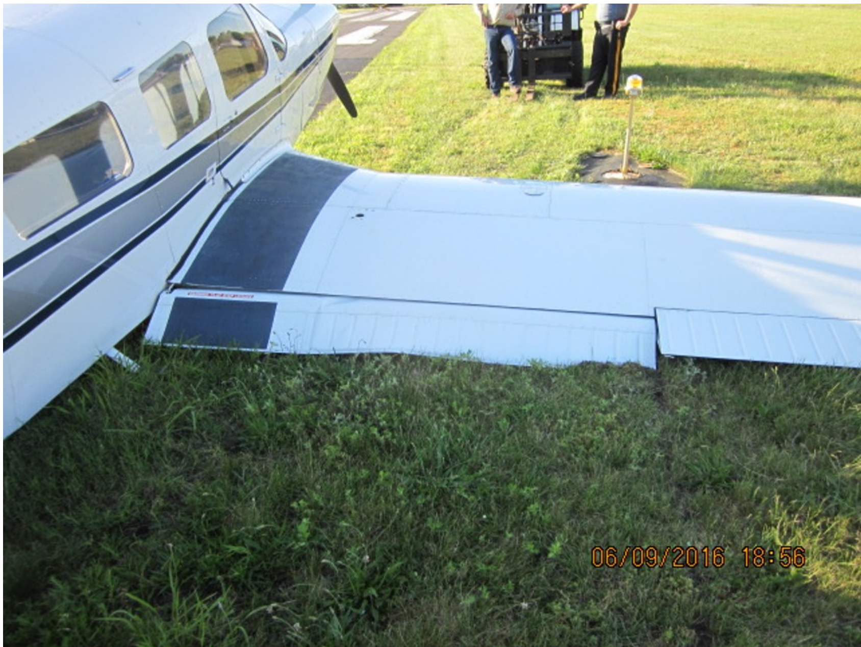
Photo 1 – View of damage to right wing flap (Courtesy of FAA)
