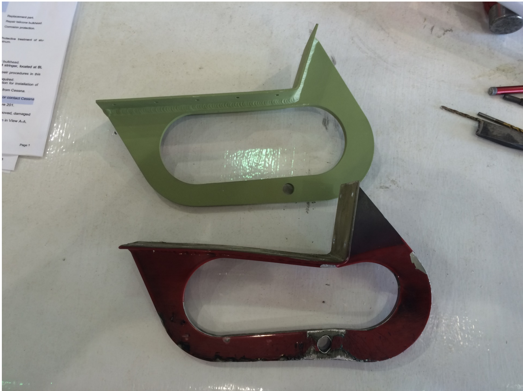
Photo 2 – Comparison of Damaged Tail Hook vs. New Tail Hook (Photo Courtesy of FAA)
