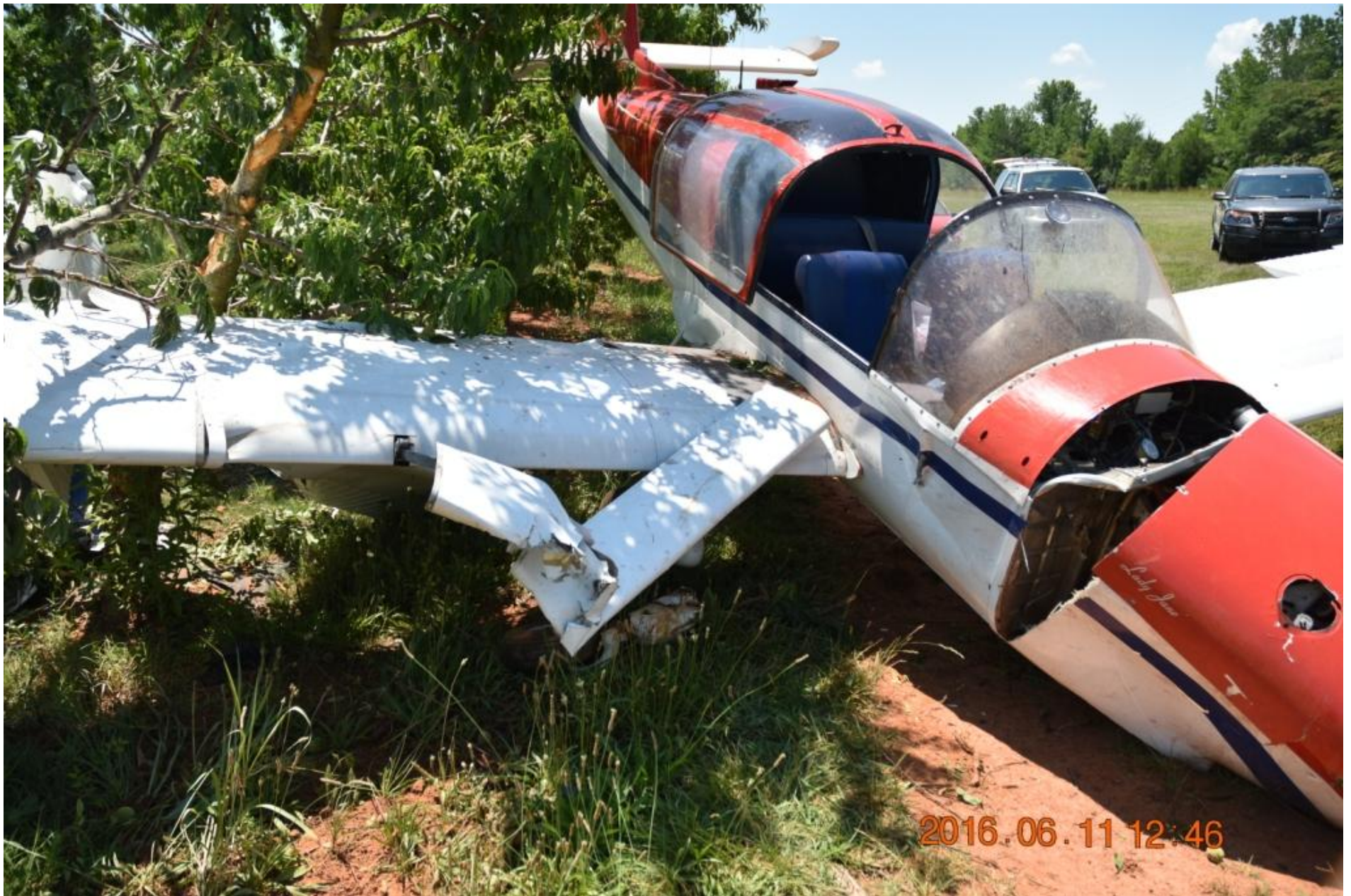
Photo 1 – View of right wing damage (photo courtesy of the FAA)
